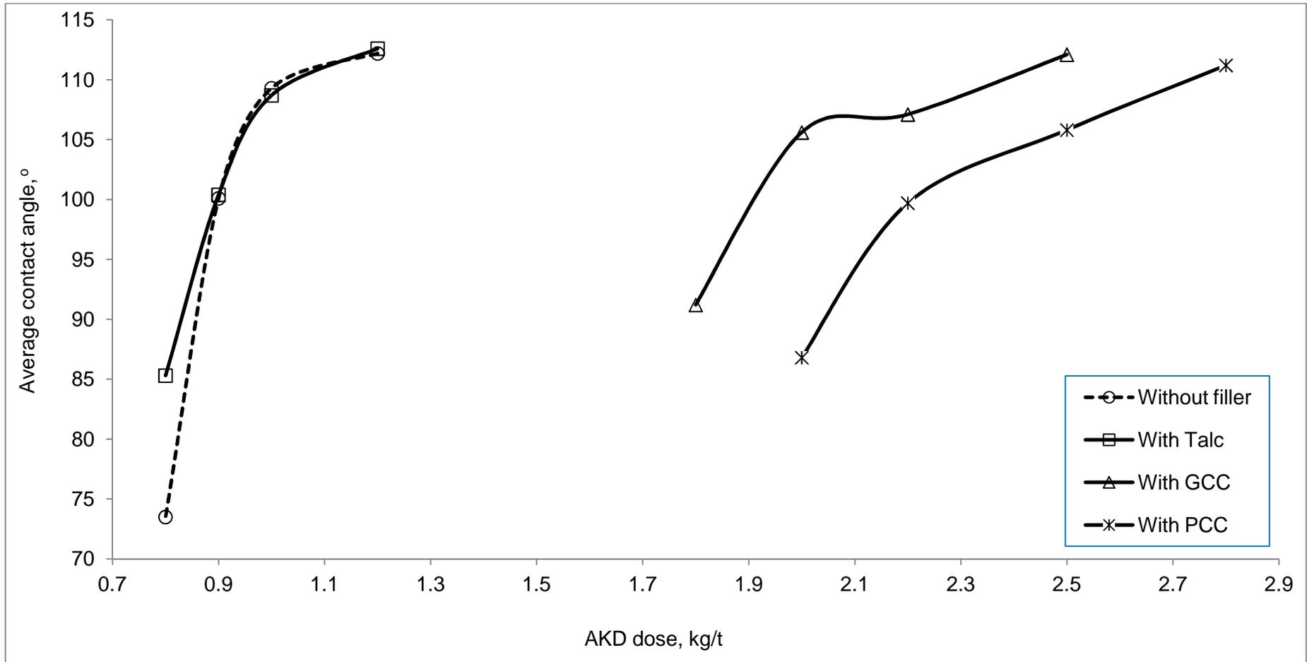
Figure 6: Effect of filler on contact angle with MHW pulp in AKD sizing
