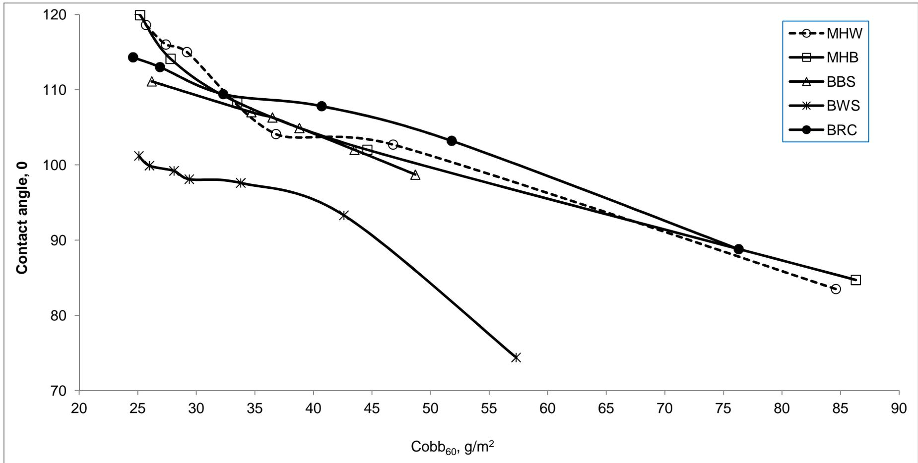
Figure 59: Cobb vs. contact angle relationship for different pulp furnishes in ASA sizing with GCC filler
