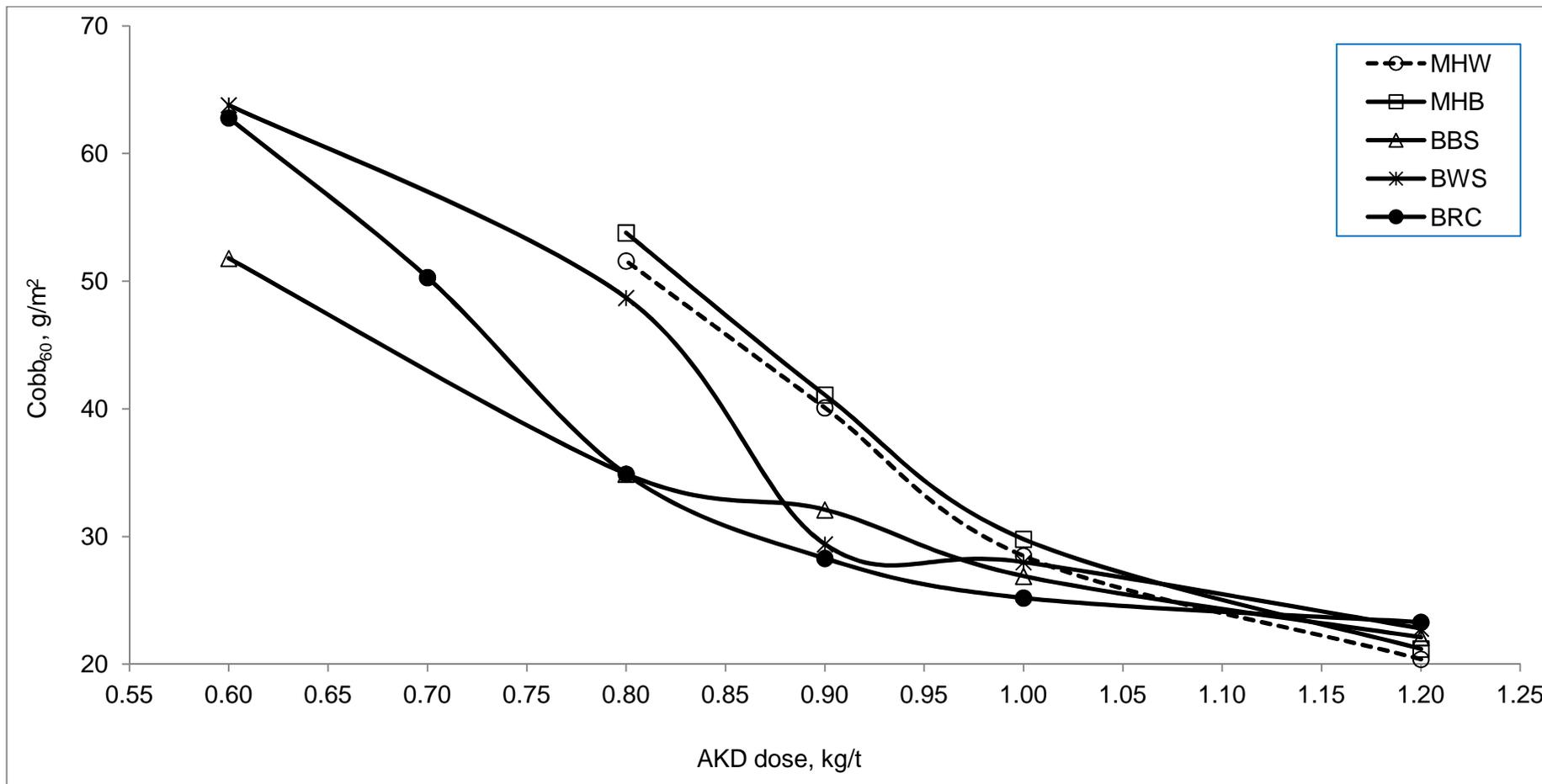
Figure 21: Comparison of Cobb<sub>60</sub> value of different pulp furnishes in AKD sizing with talc filler
