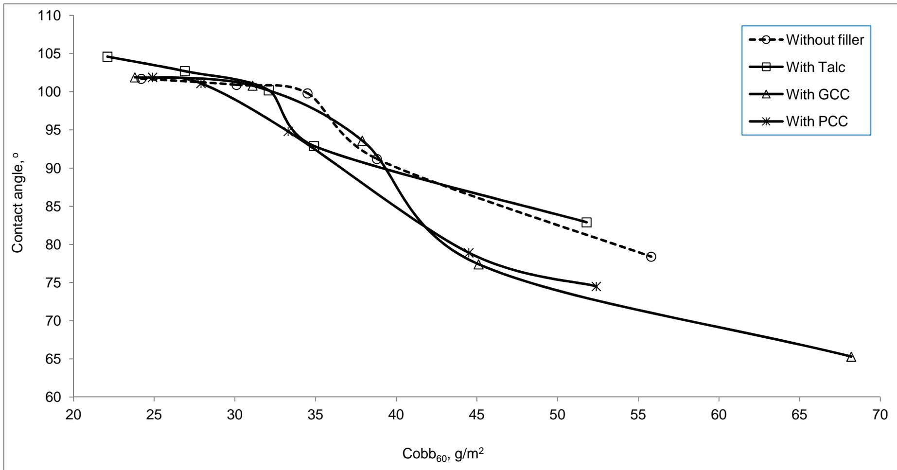
Figure 13: Cobb<sub>60</sub> vs. contact angle relationship for BBS pulp in AKD sizing
