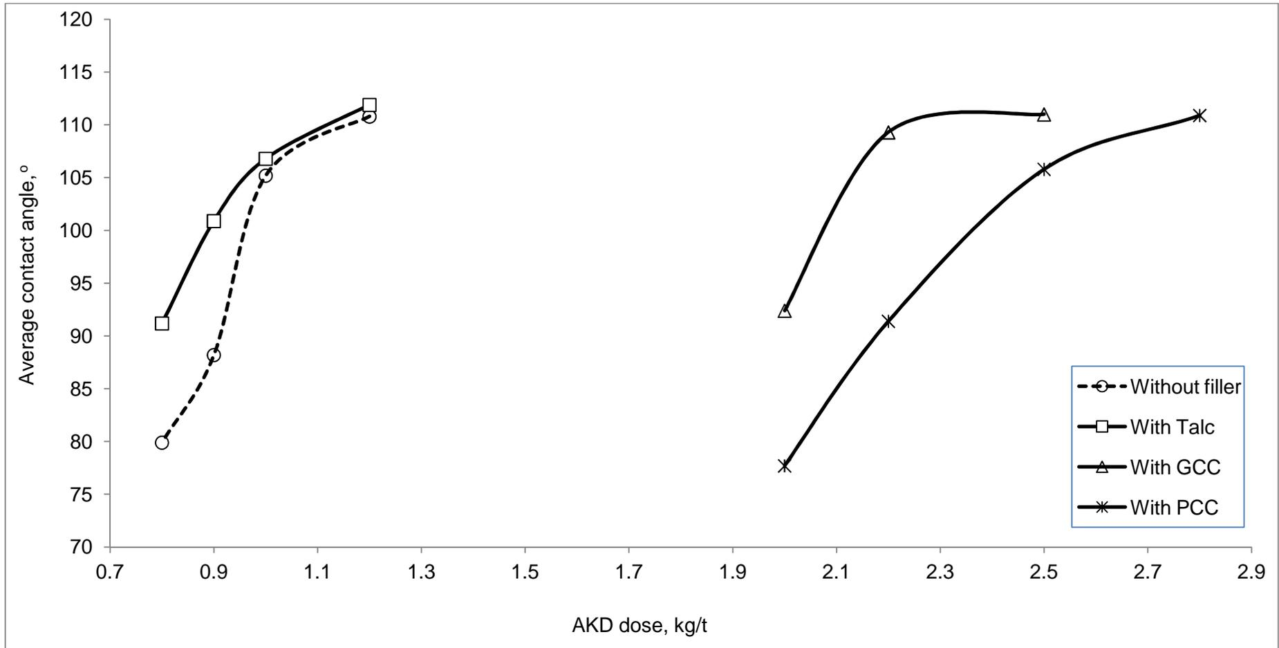
Figure 9: Effect of filler on contact angle with MHB pulp in AKD sizing
