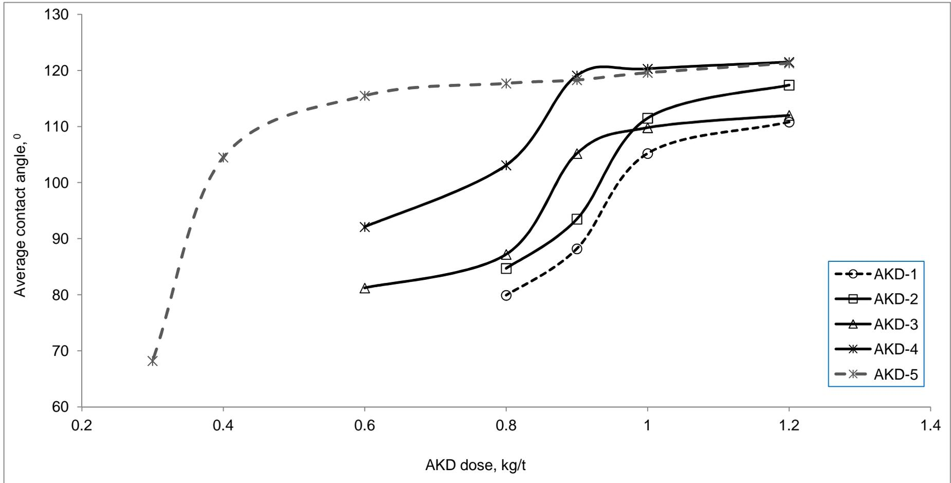
Figure 2: Comparison of contact angle of paper prepared from MHB pulp with different AKD emulsions
