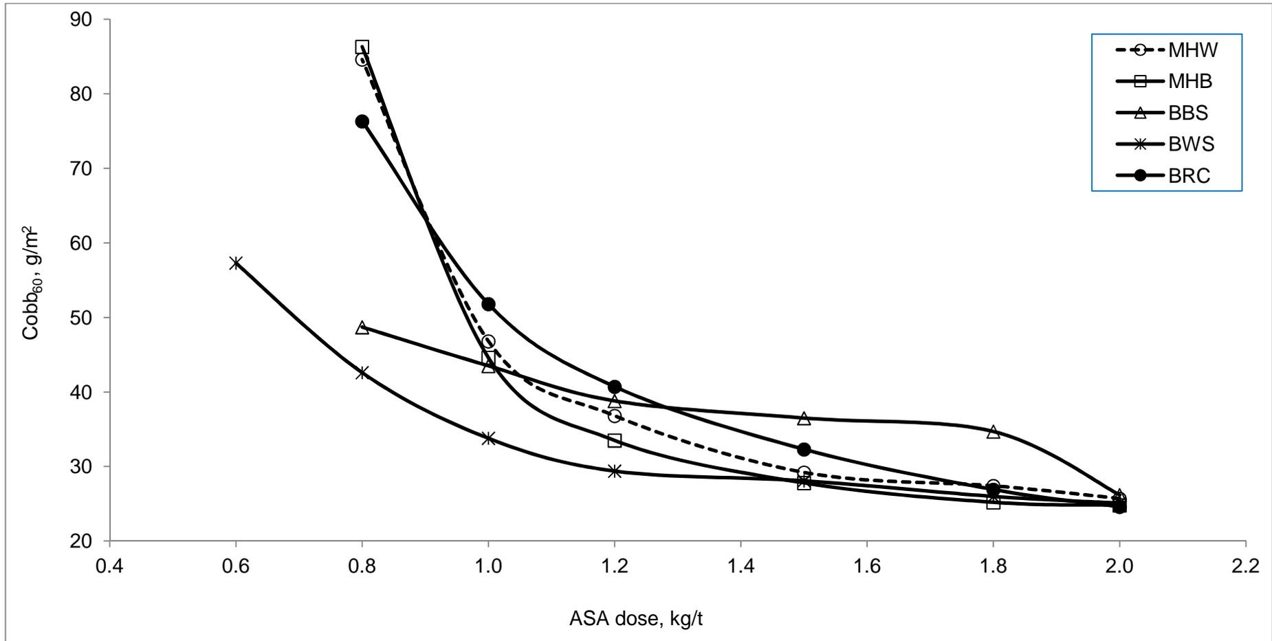
Figure 51: Comparison of Cobb<sub>60</sub> value of different pulp furnishes in ASA sizing with GCC filler
