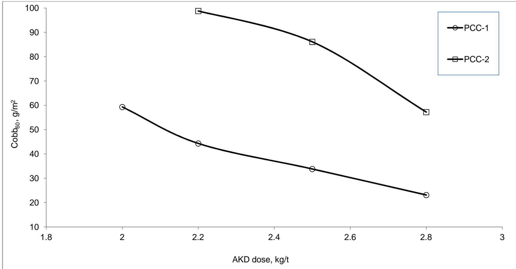
Figure 4: Effect of PCC filler on Cobb<sub>60</sub> value of paper made with MHW pulp in AKD sizing
