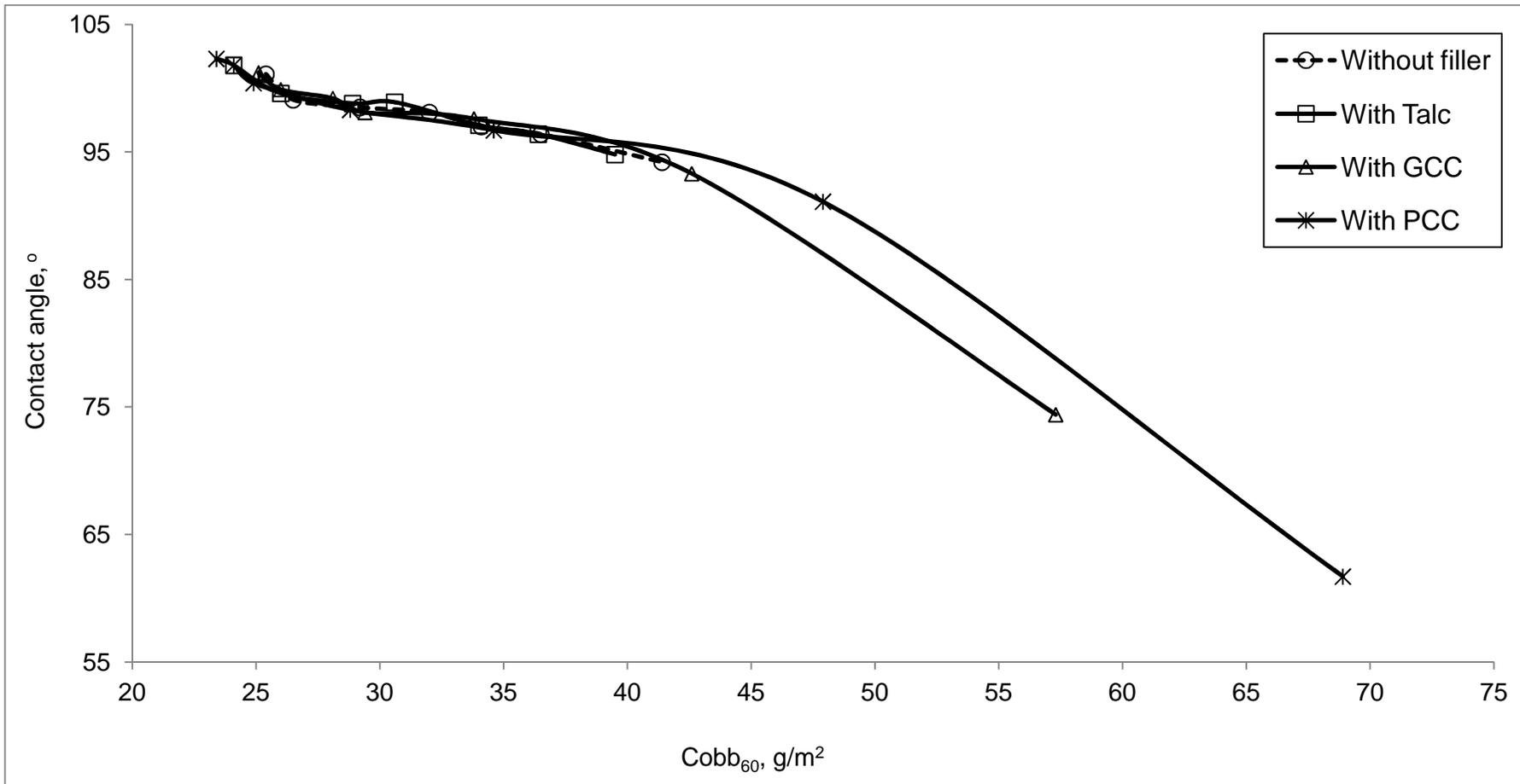
Table 45: Cobb<sub>60</sub> vs. contact angle relationship of BWS pulp in ASA sizing with different fillers
