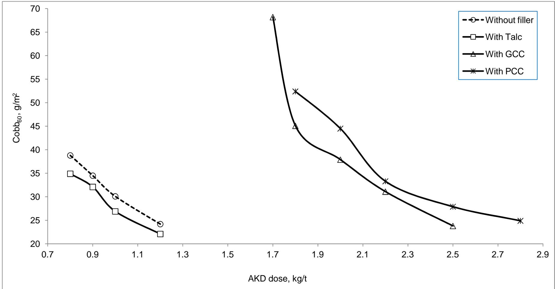
Figure 11: Effect of filler on Cobb<sub>60</sub> value with BBS pulp in AKD sizing
