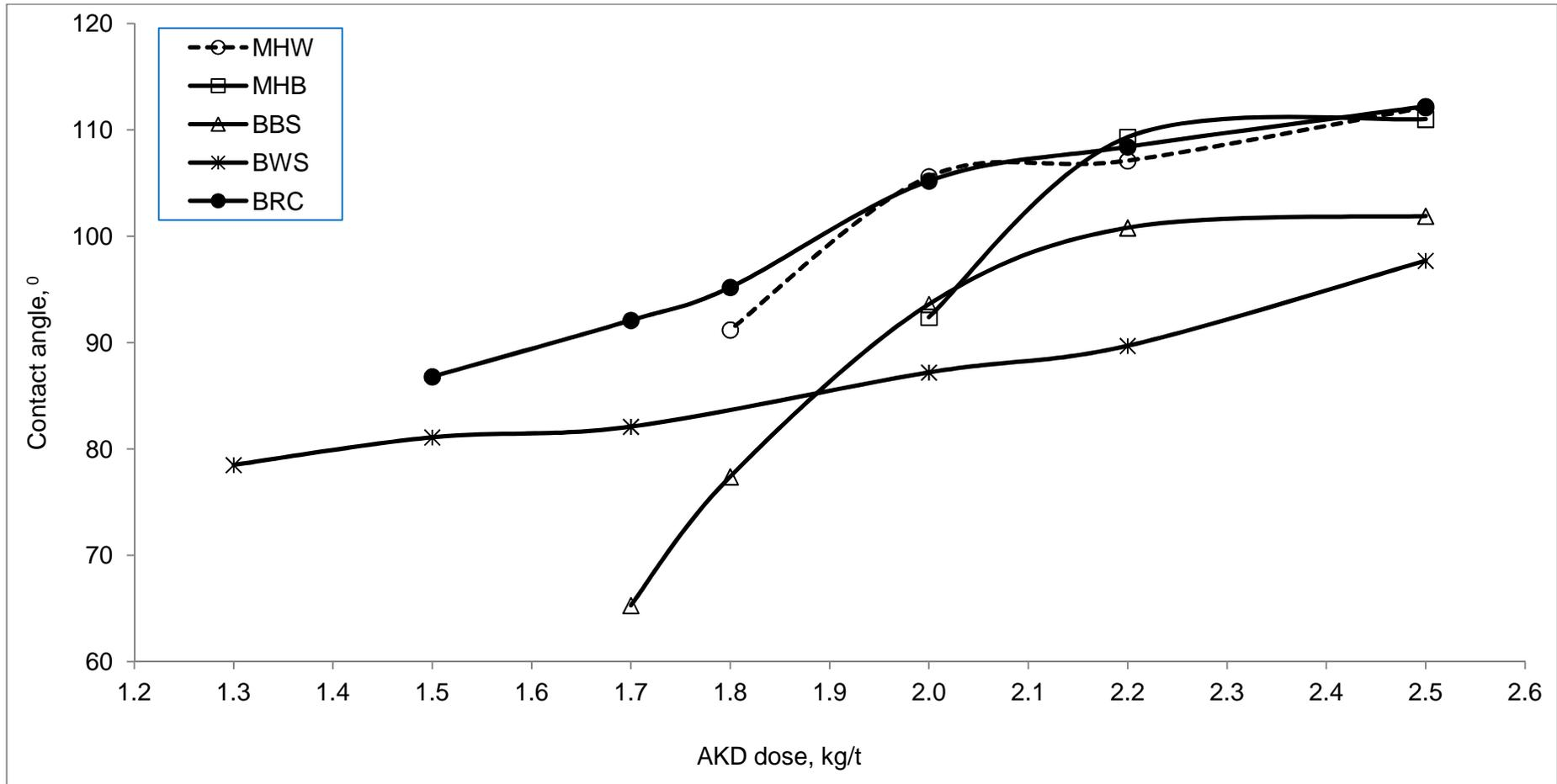
Figure 26: Comparison of contact angle of different pulp furnishes in AKD sizing with GCC filler
