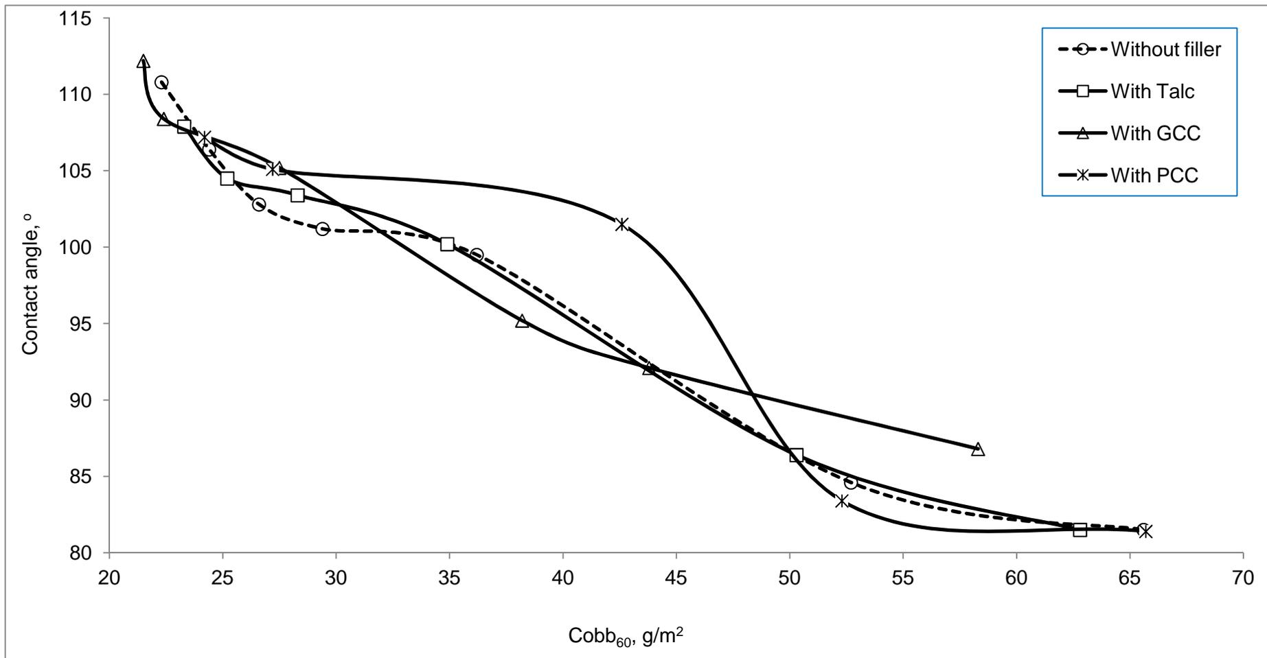
Figure 19: Cobb<sub>60</sub> vs. contact angle relationship for BRC pulp in AKD sizing
