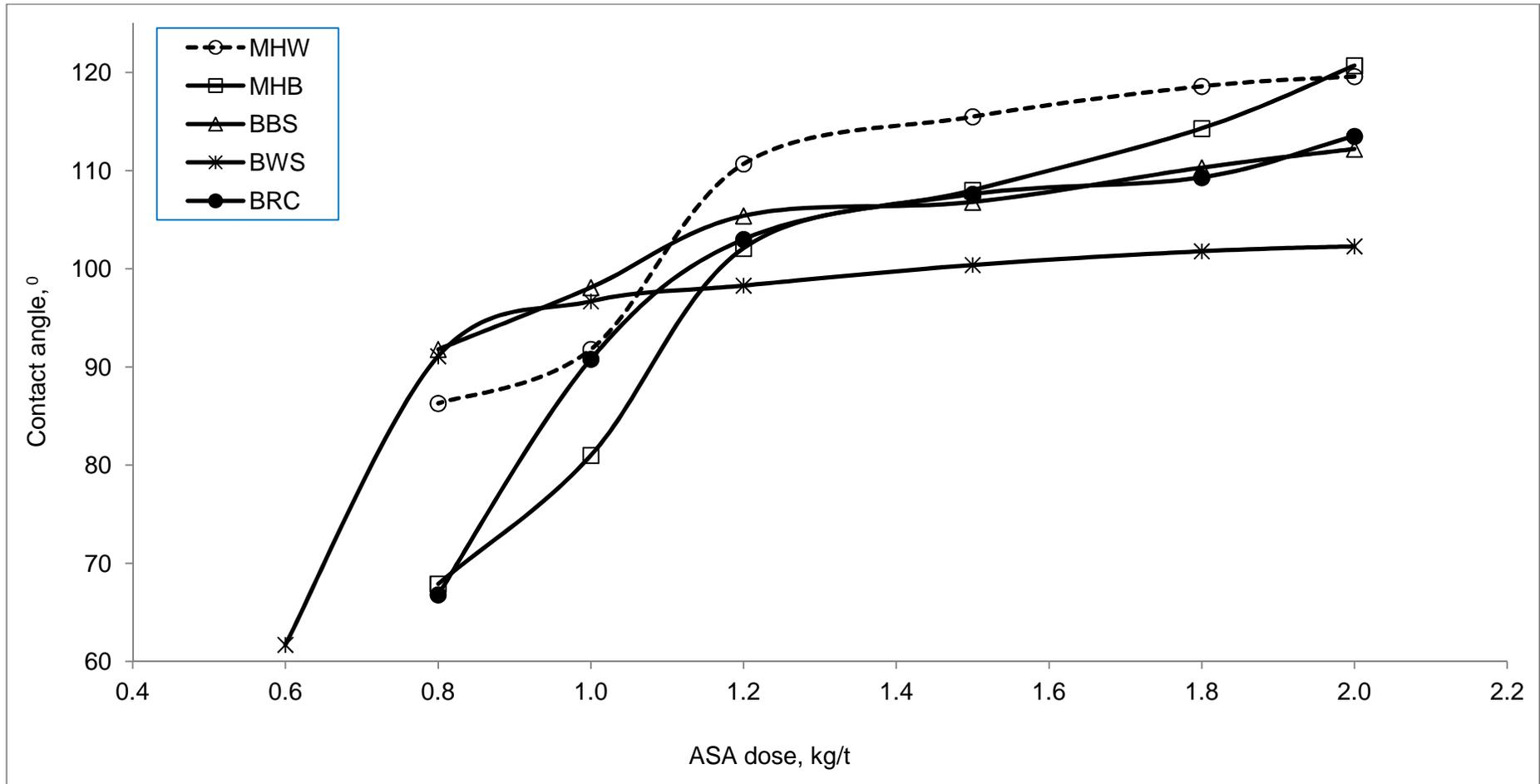
Figure 56: Comparison of contact angle of different pulp furnishes in ASA sizing with PCC filler
