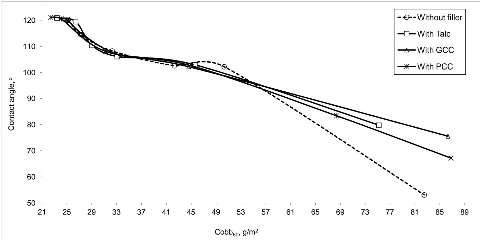
Table 36: Cobb<sub>60</sub> vs. contact angle relationship of MHB pulp in ASA sizing with different fillers
