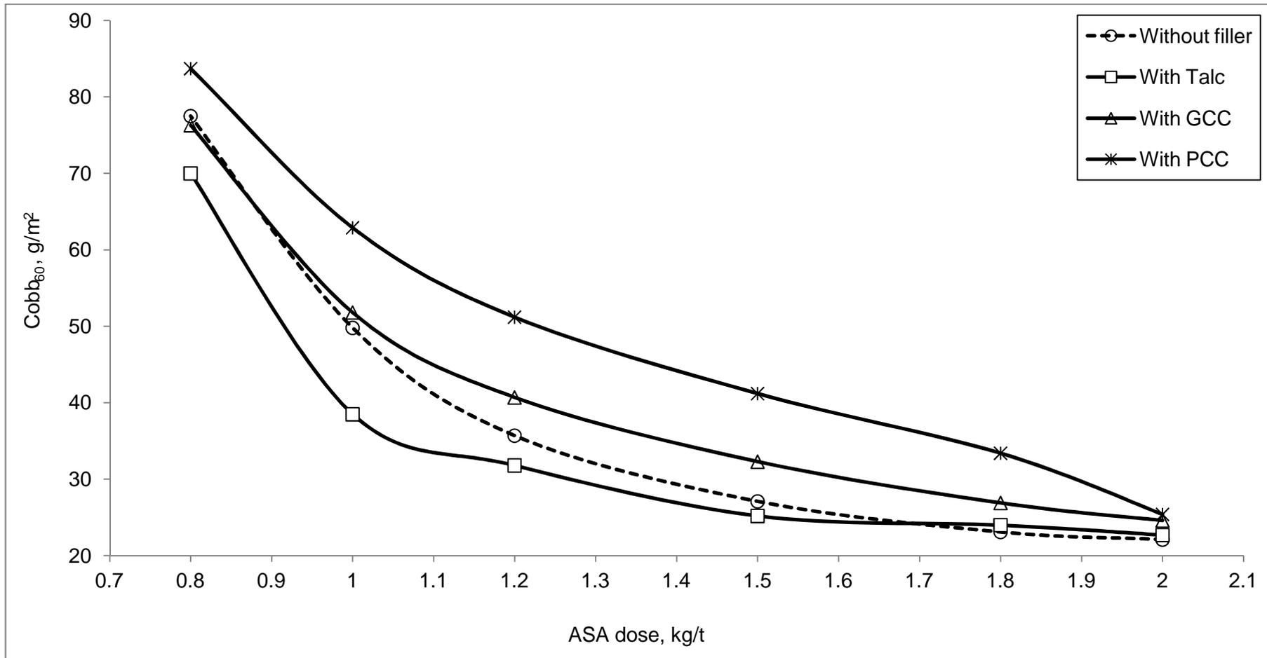
Figure 46: Effect of filler on Cobb<sub>60</sub> value with BRC pulp in ASA sizing
