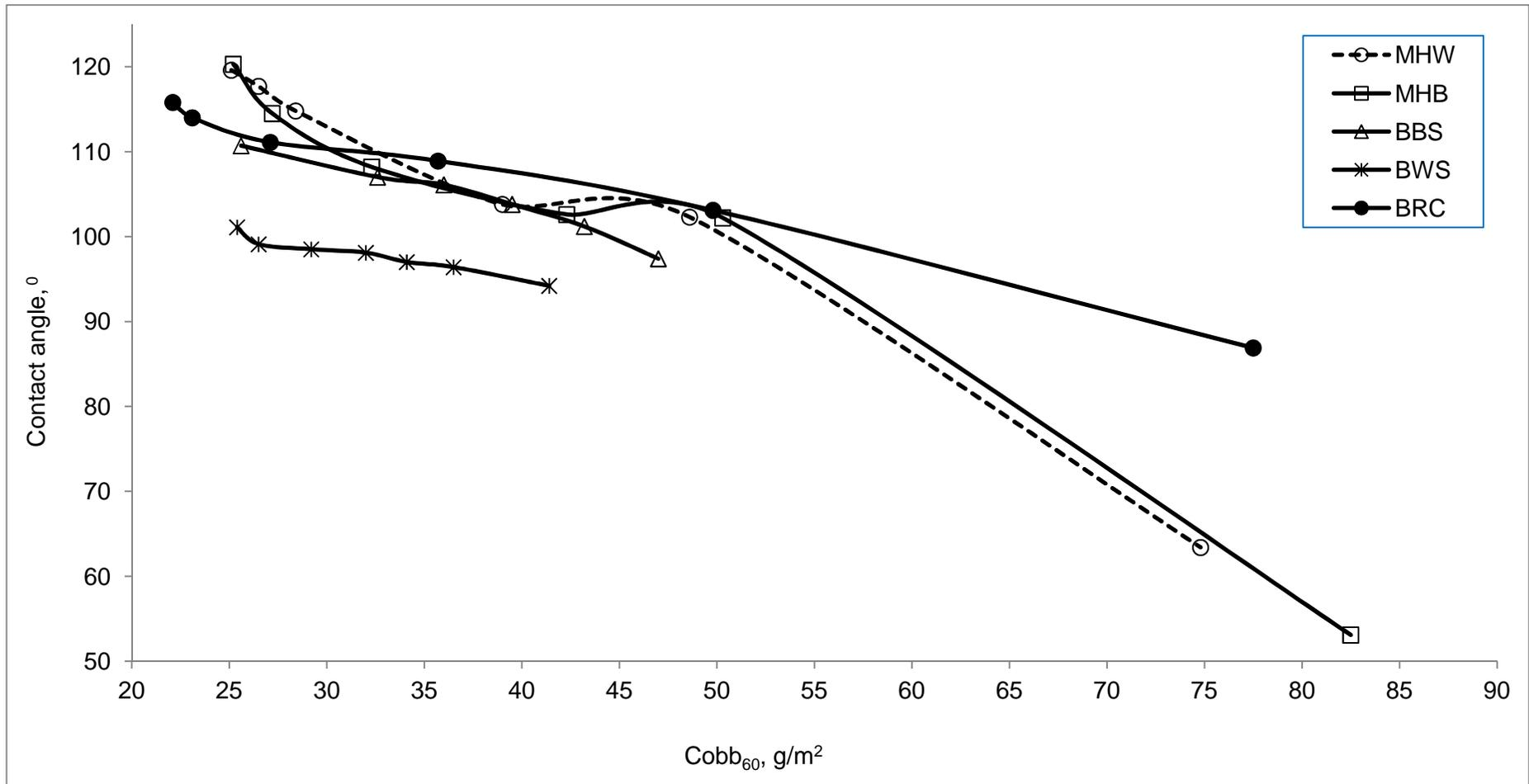
Figure 57: Cobb<sub>60</sub> vs. contact angle relationship for different pulp furnishes in ASA sizing (without Filler)
