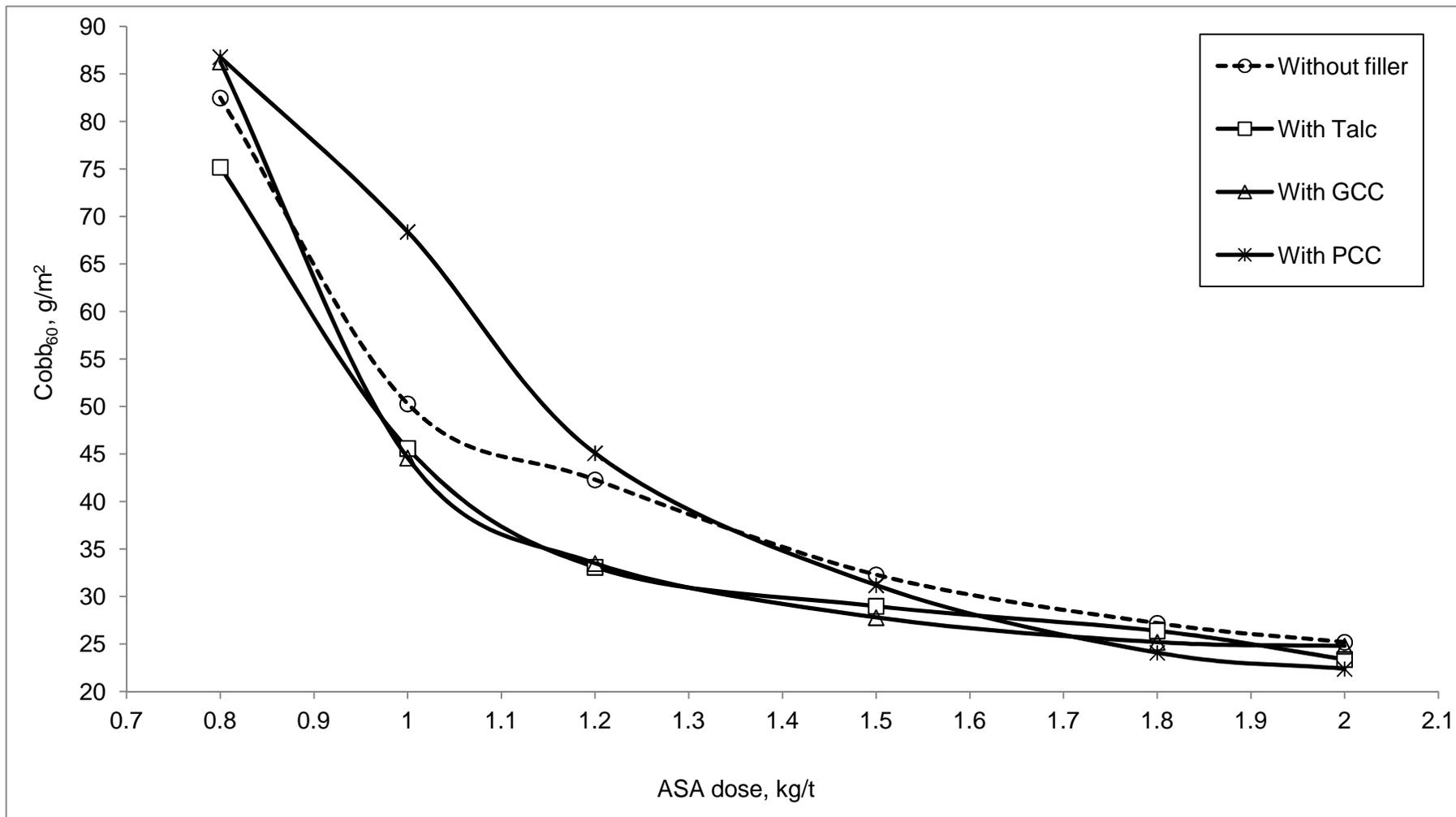
Figure 34: Effect of filler on Cobb<sub>60</sub> value with MHB pulp in ASA sizing
