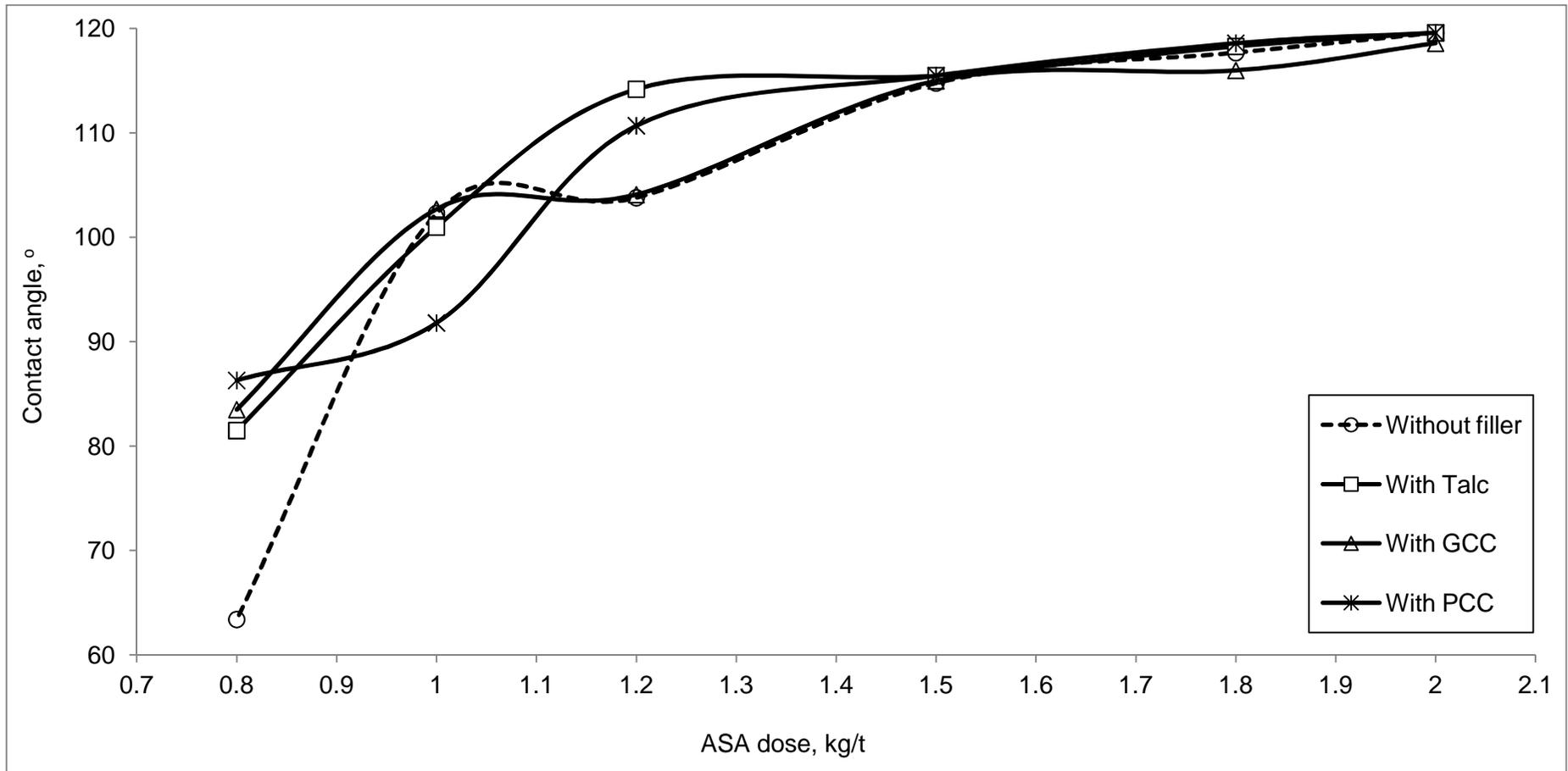
Figure 38: Effect of filler on contact angle with MHW pulp in ASA sizing
