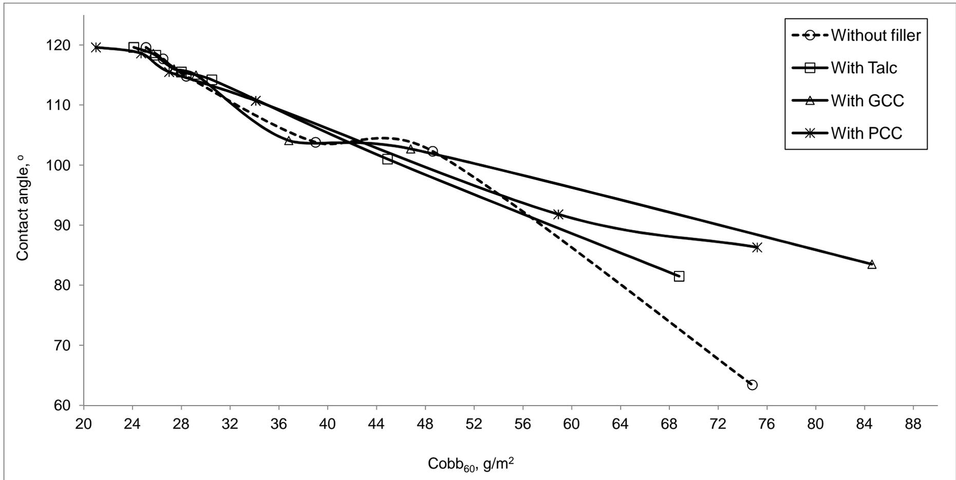
Table 39: Cobb<sub>60</sub> vs. contact angle relationship of MHW pulp in ASA sizing with different fillers
