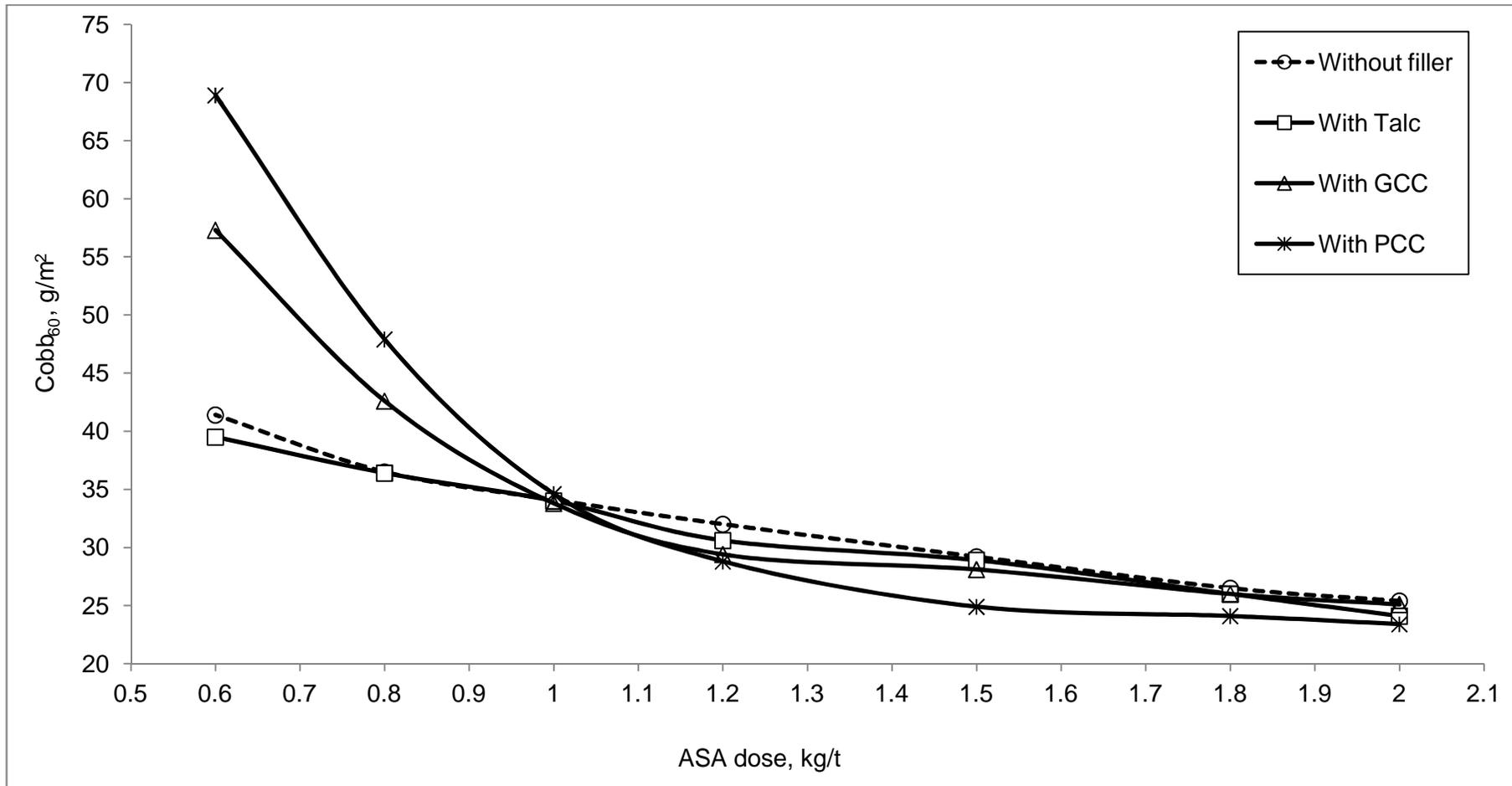
Figure 43: Effect of filler on Cobb<sub>60</sub> value with BWS pulp in ASA sizing
