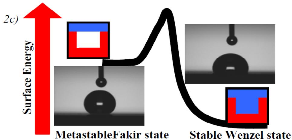
Figure:-2 Schematic drawing to show the energy barrier that stabilizes the metastable Fakir state (2)
