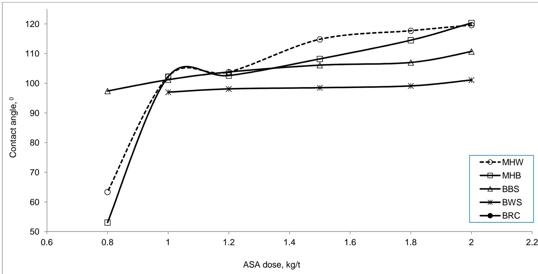
Figure 53: Comparison of contact angle of different pulp furnishes in ASA sizing (without filler)
