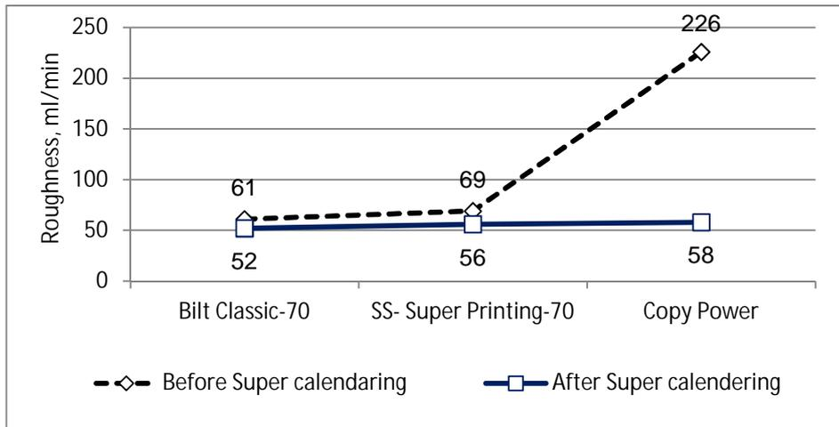
Figure 3. Effect of super calendering on felt side of paper
