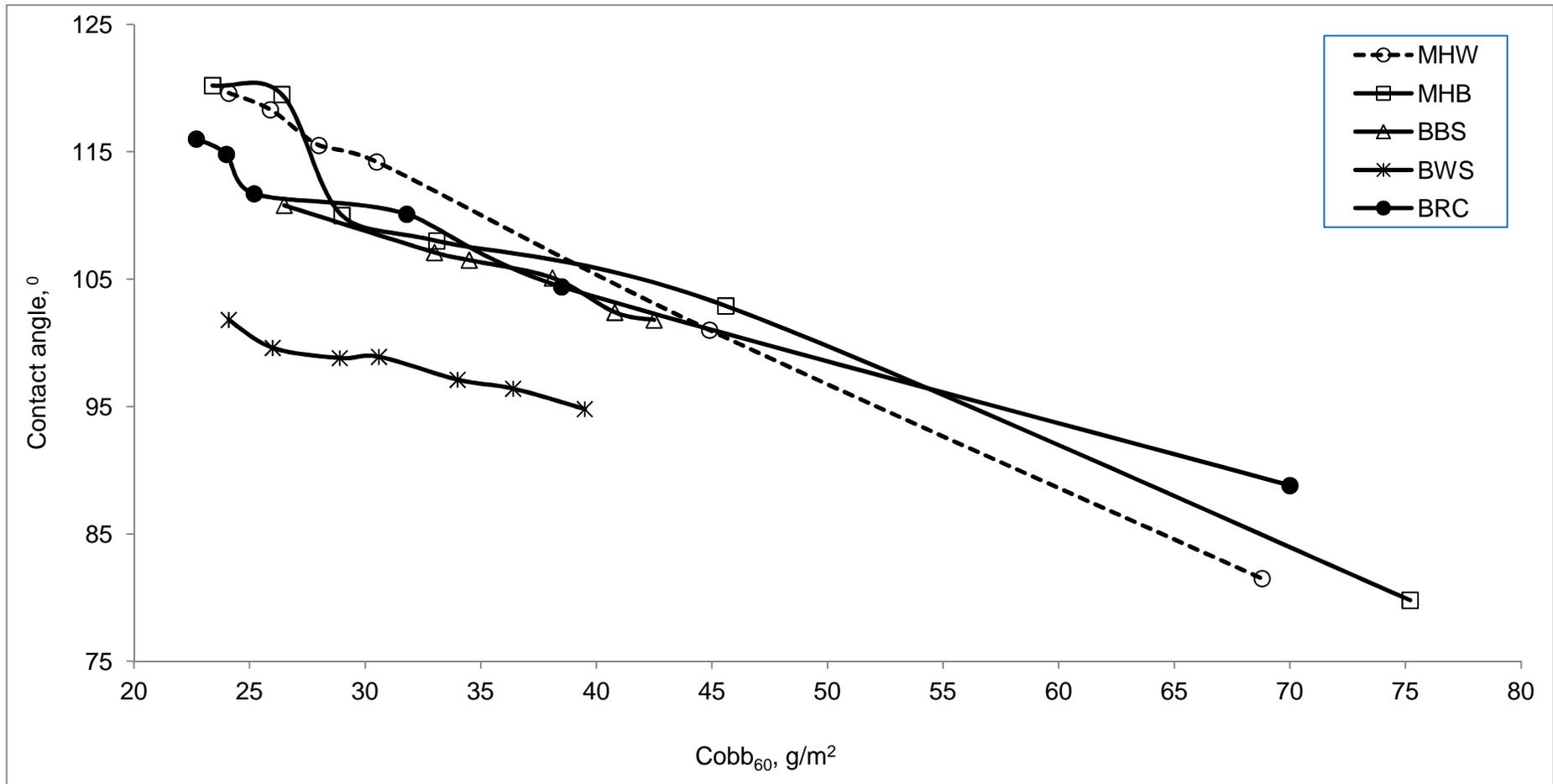
Figure 58: Cobb vs. contact angle relationship for different pulp furnishes in ASA sizing with talc filler
