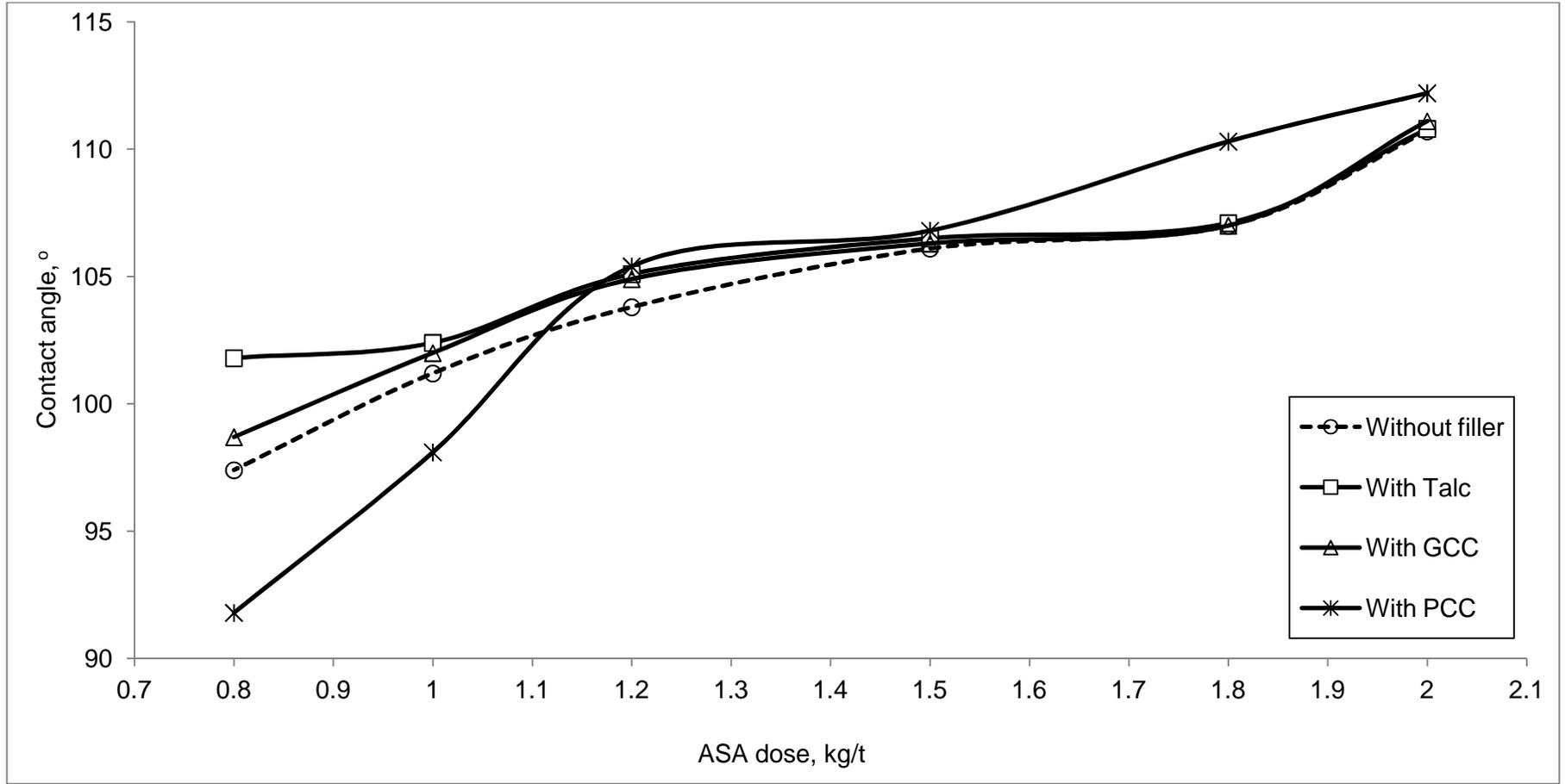
Figure 41: Effect of filler on contact angle with BBS pulp in ASA sizing
