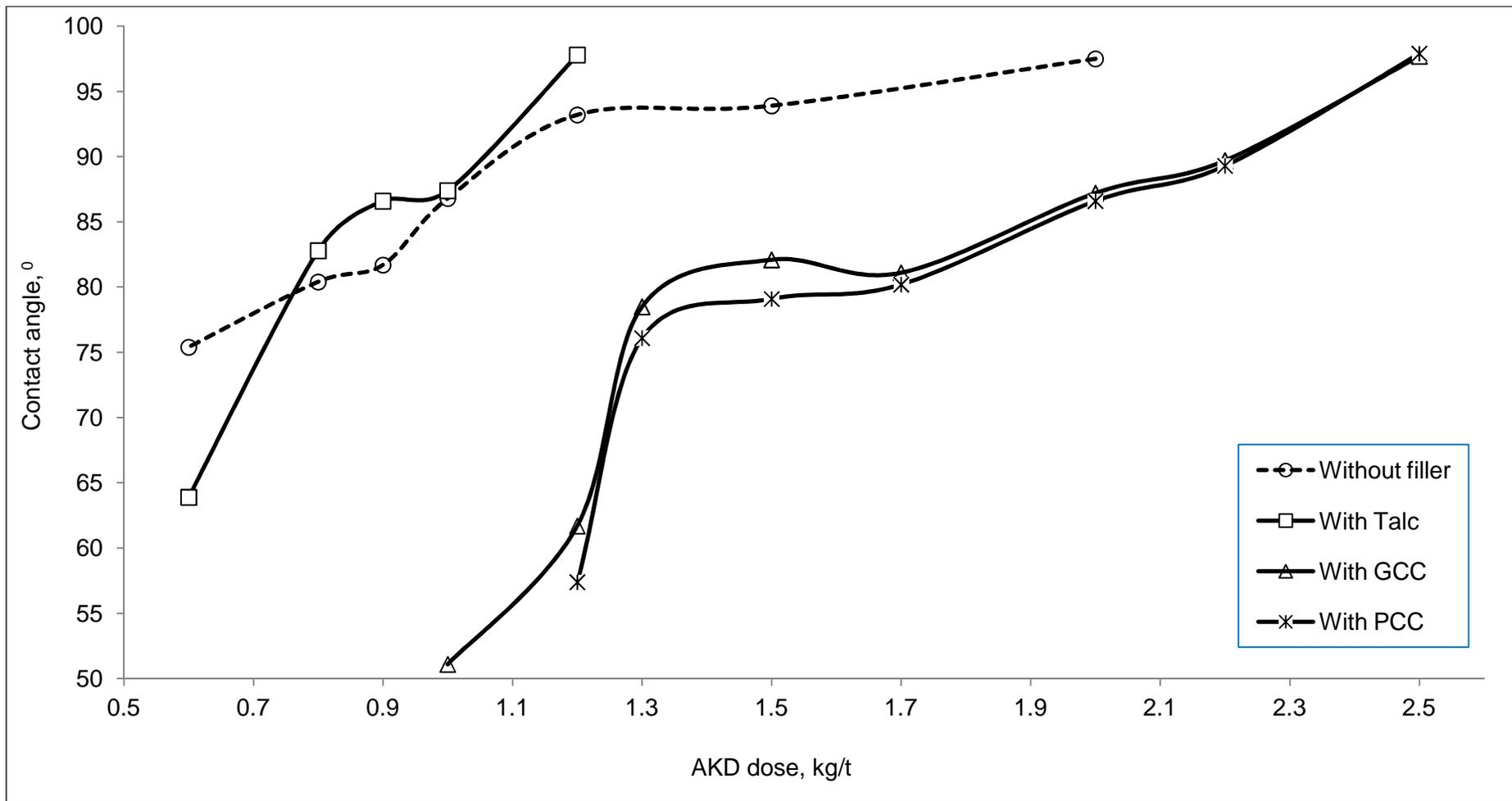
Figure 15: Effect of filler on contact angle with BWS pulp in AKD sizing
