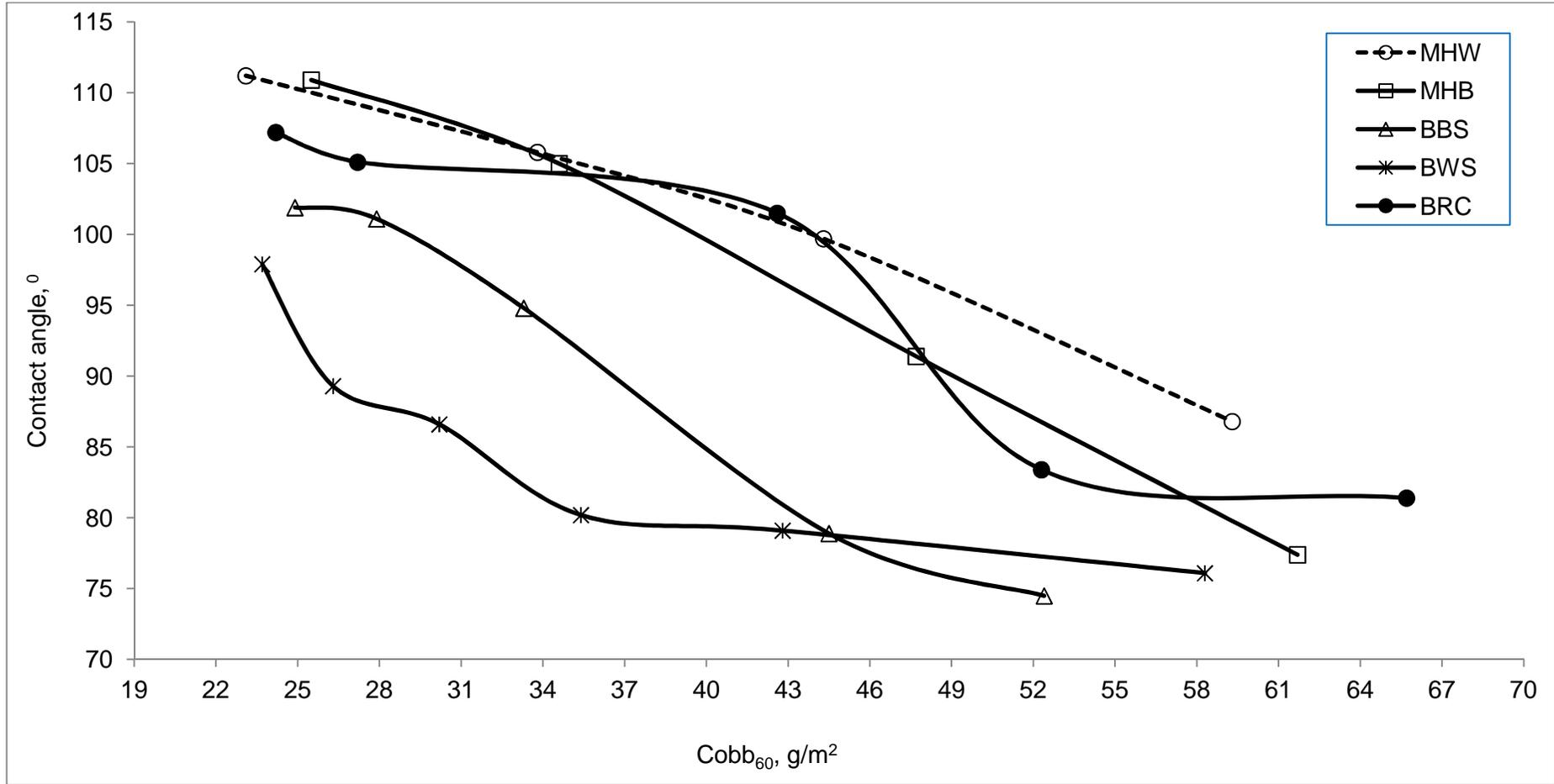
Figure 31: Cobb vs. contact angle relationship for different pulp furnishes in AKD sizing with PCC filler
