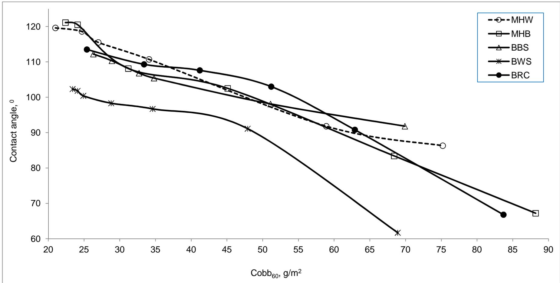
Figure 60: Cobb vs. contact angle relationship for different pulp furnishes in ASA sizing with PCC filler
