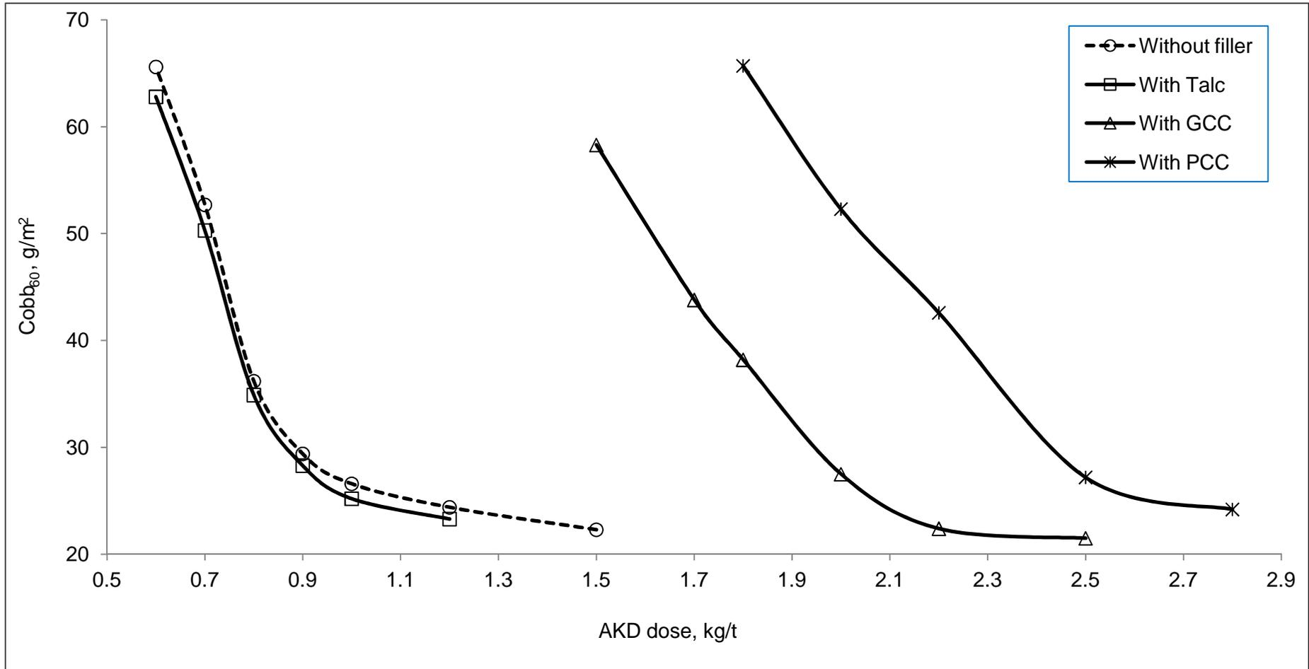
Figure 17: Effect of filler on Cobb<sub>60</sub> value with BRC pulp in AKD sizing
