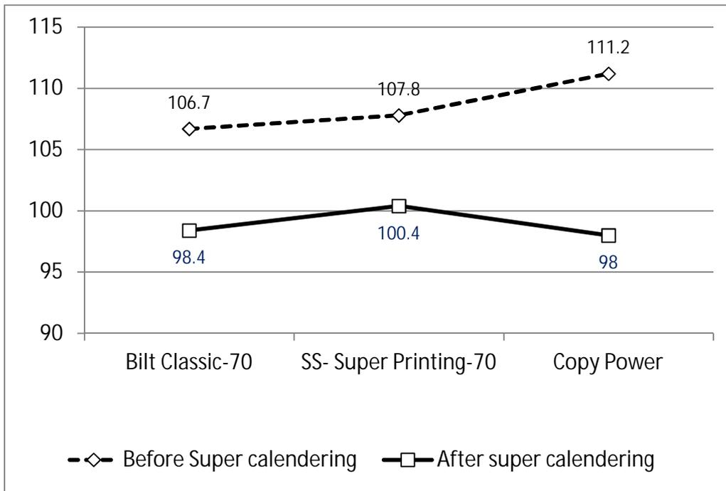
Figure 5. Effect of super calendering on contact angle of felt side of paper
