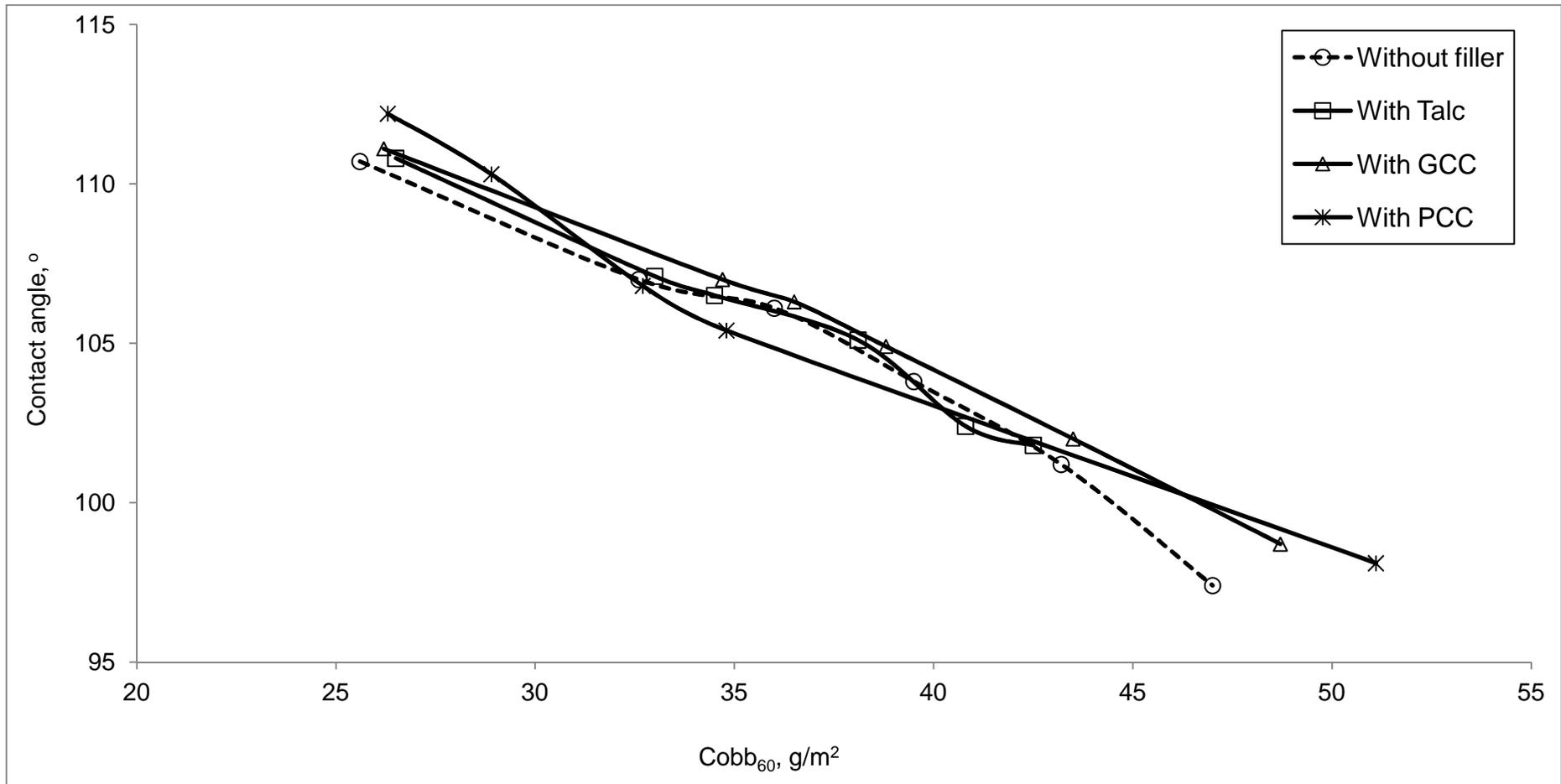
Table 42: Cobb<sub>60</sub> vs. contact angle relationship of BBS pulp in ASA sizing with different fillers
