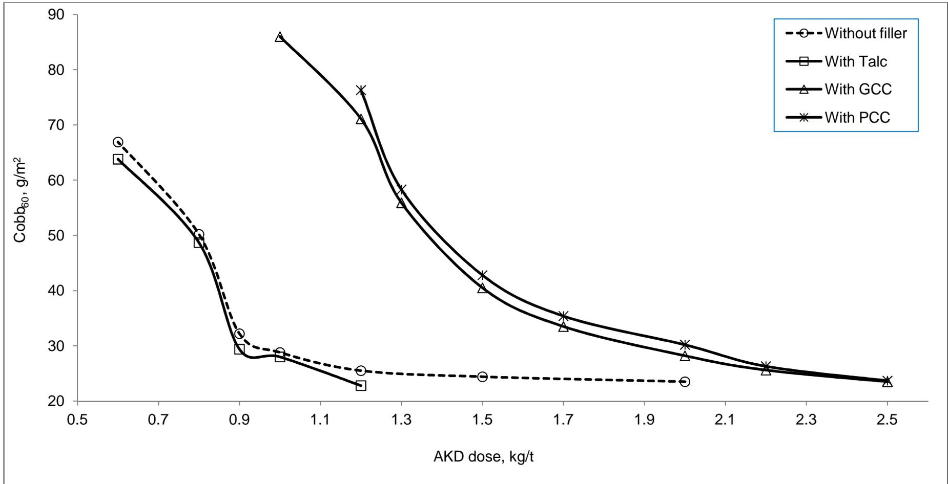
Figure 14: Effect of filler on Cobb<sub>60</sub> value with BWS pulp in AKD sizing
