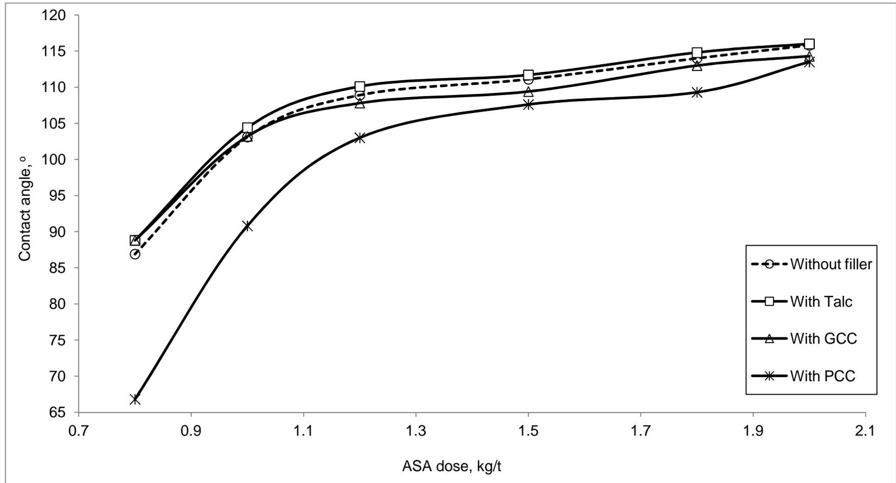
Figure 47: Effect of filler on contact angle with BRC pulp in ASA sizing
