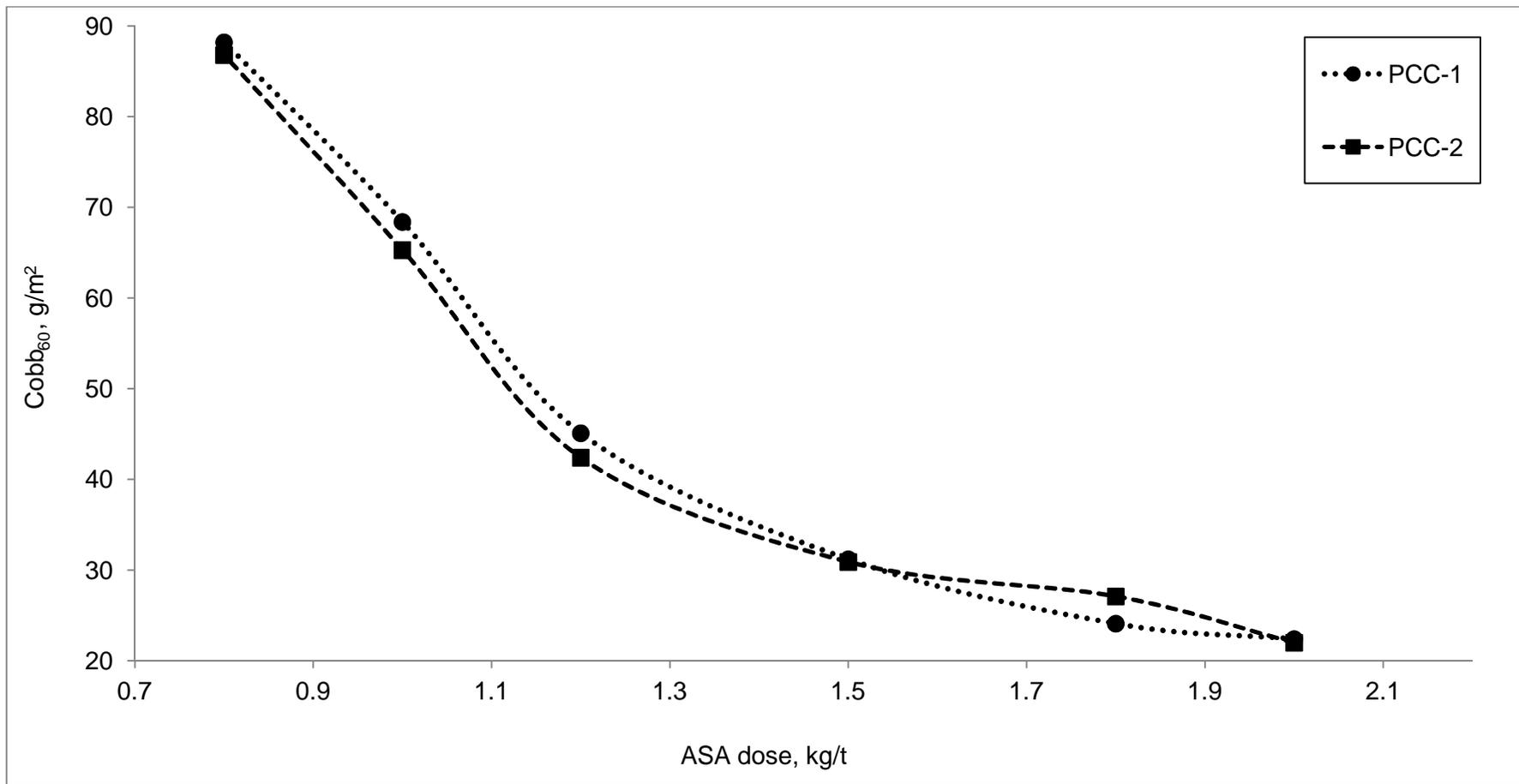
Figure 33: Sizing performance of different PCC fillers with MHB pulp in ASA sizing
