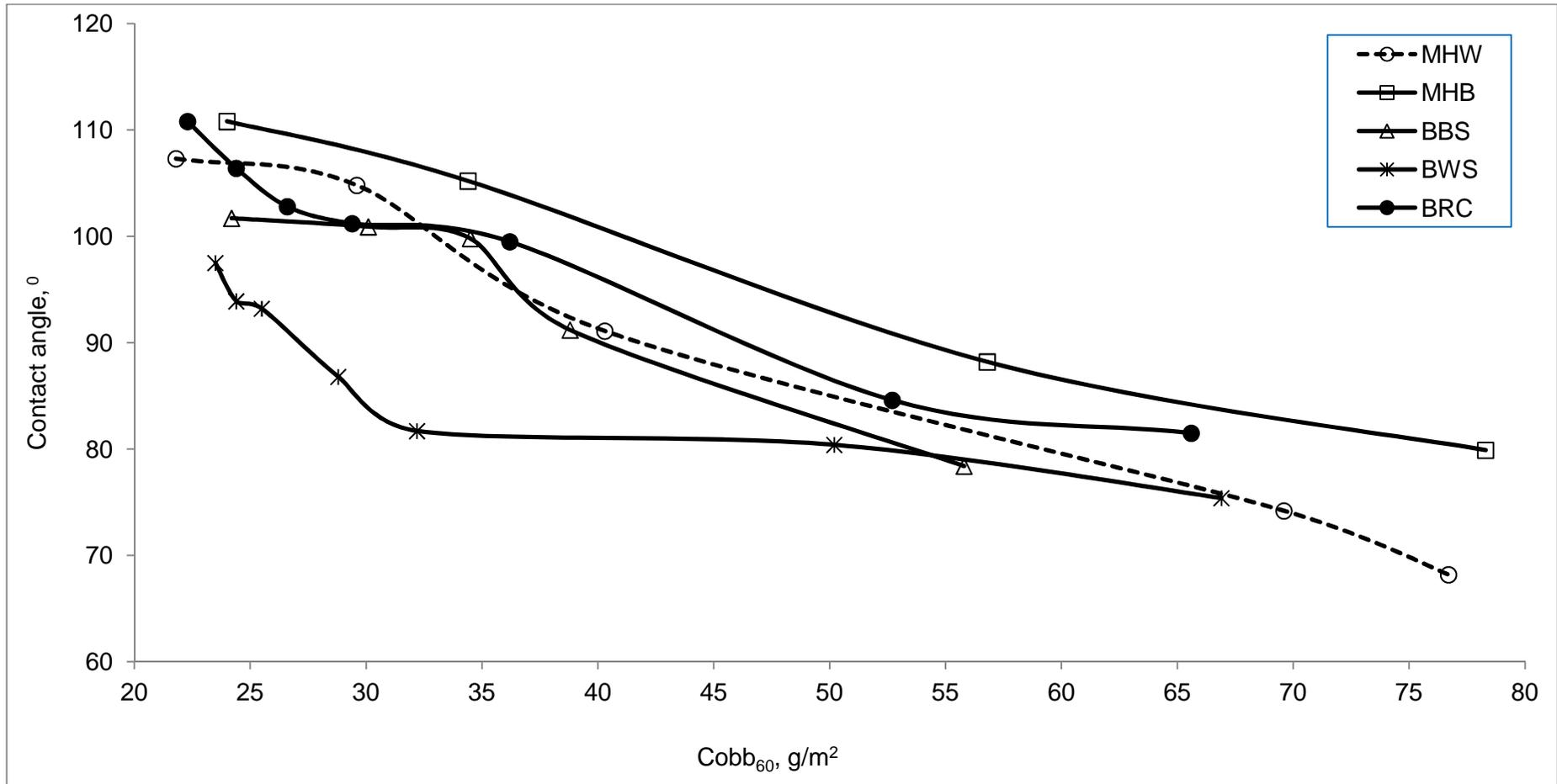
Figure 28: Cobb<sub>60</sub> vs. contact angle relationship for different pulp furnishes in AKD sizing (without Filler)
