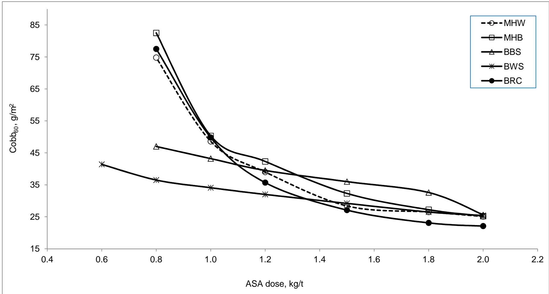
Figure 49: Comparison of Cobb<sub>60</sub> value of different pulp furnishes in ASD sizing (without filler)
