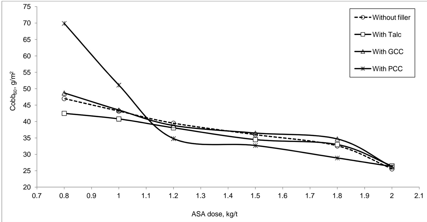
Figure 40: Effect of filler on Cobb<sub>60</sub> value with BBS pulp in ASA sizing
