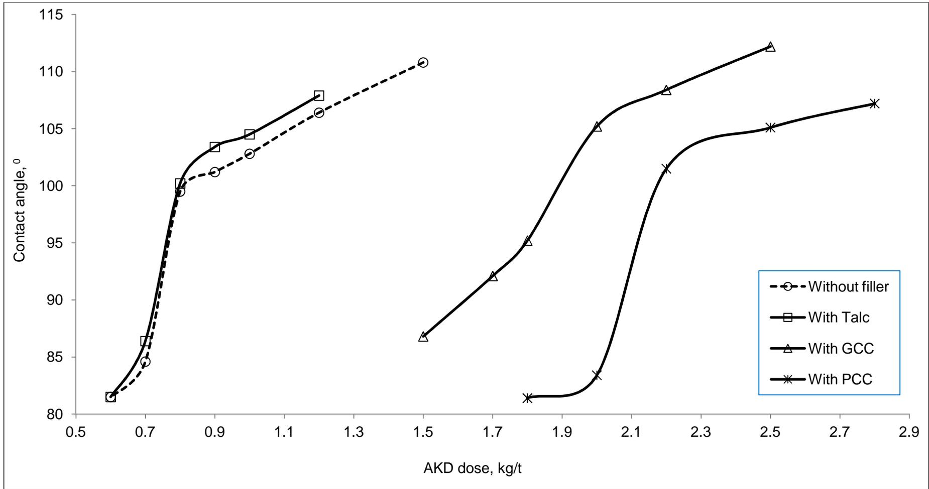
Figure 18: Effect of filler on contact angle with BRC pulp in AKD sizing
