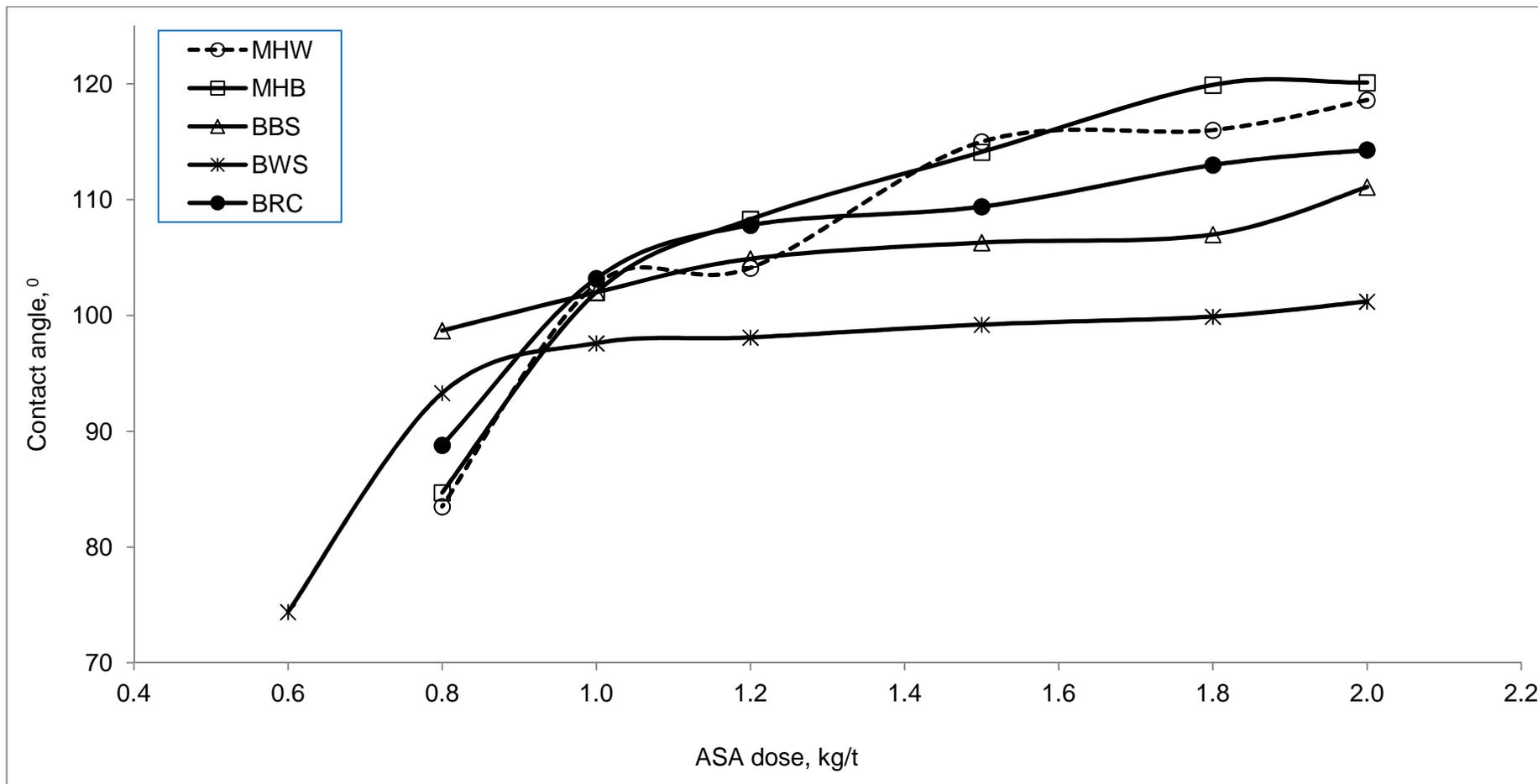
Figure 55: Comparison of contact angle of different pulp furnishes in ASA sizing with GCC filler
