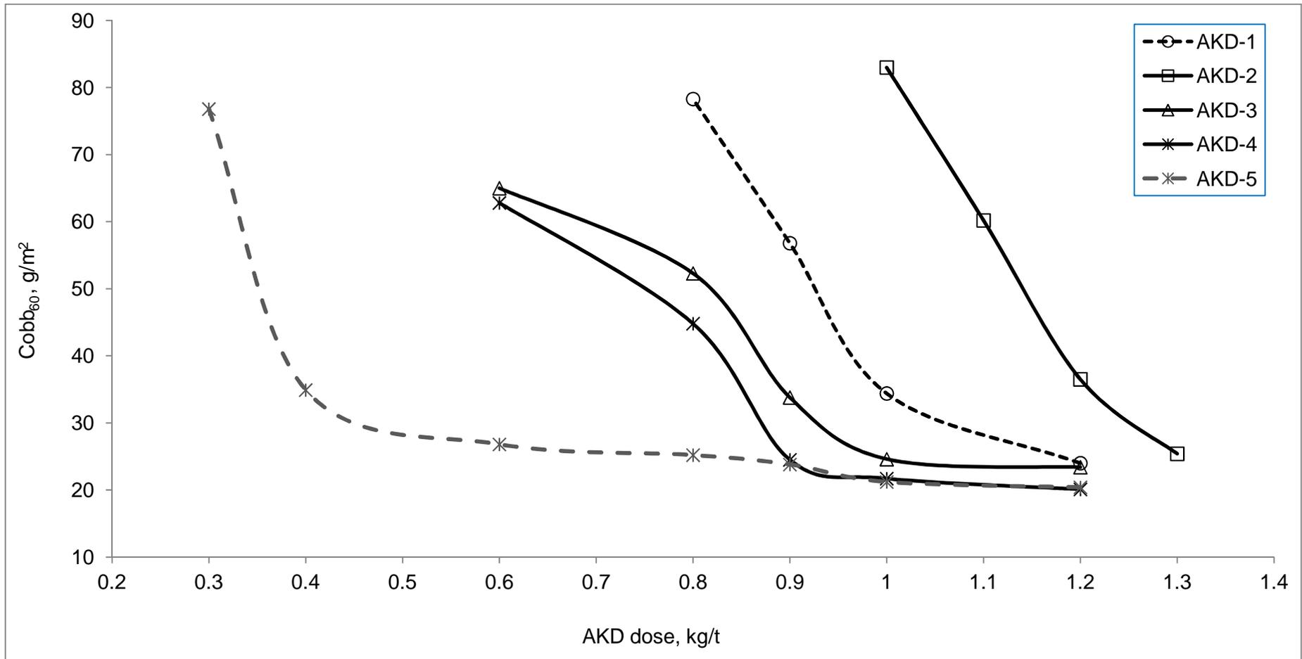
Figure 1: Comparison of Cobb<sub>60</sub> of paper prepared from MHB pulp with different AKD emulsions
