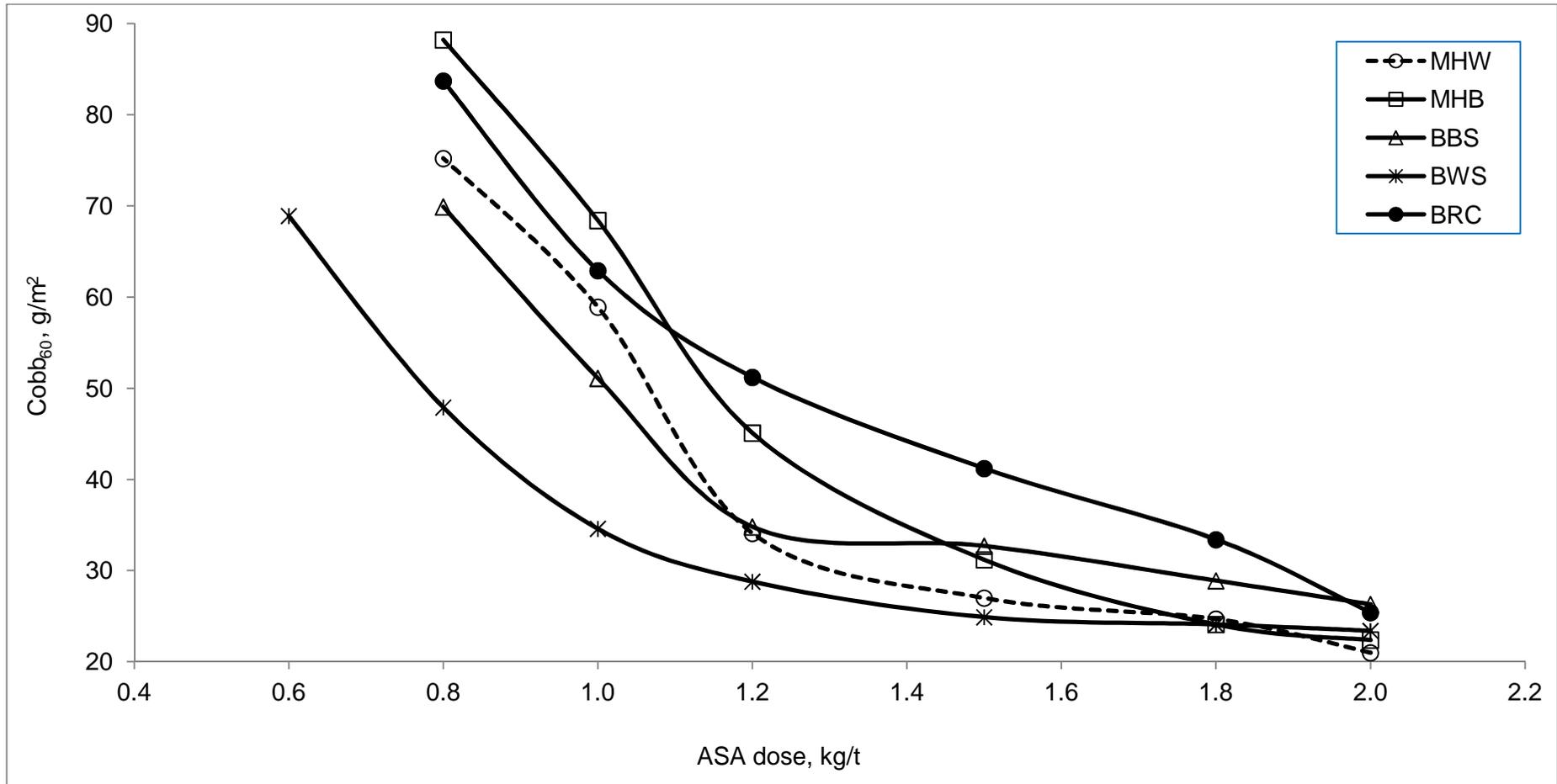
Figure 52: Comparison of Cobb<sub>60</sub> value of different pulp furnishes in ASA sizing with PCC filler
