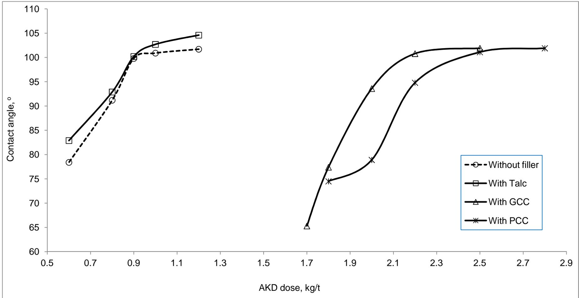
Figure 12: Effect of filler on contact angle with BBS pulp in AKD sizing
