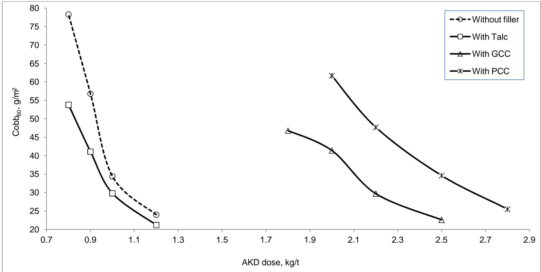
Figure 8: Effect of filler on Cobb<sub>60</sub> value with MHB pulp in AKD sizing
