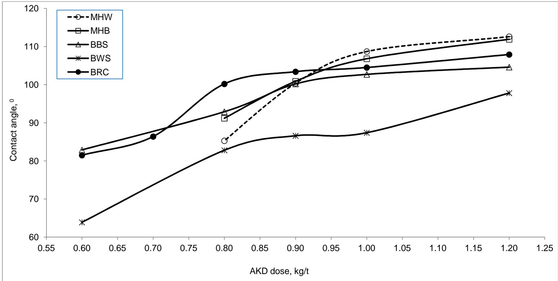
Figure 25: Comparison of contact angle of different pulp furnishes in AKD sizing with talc filler
