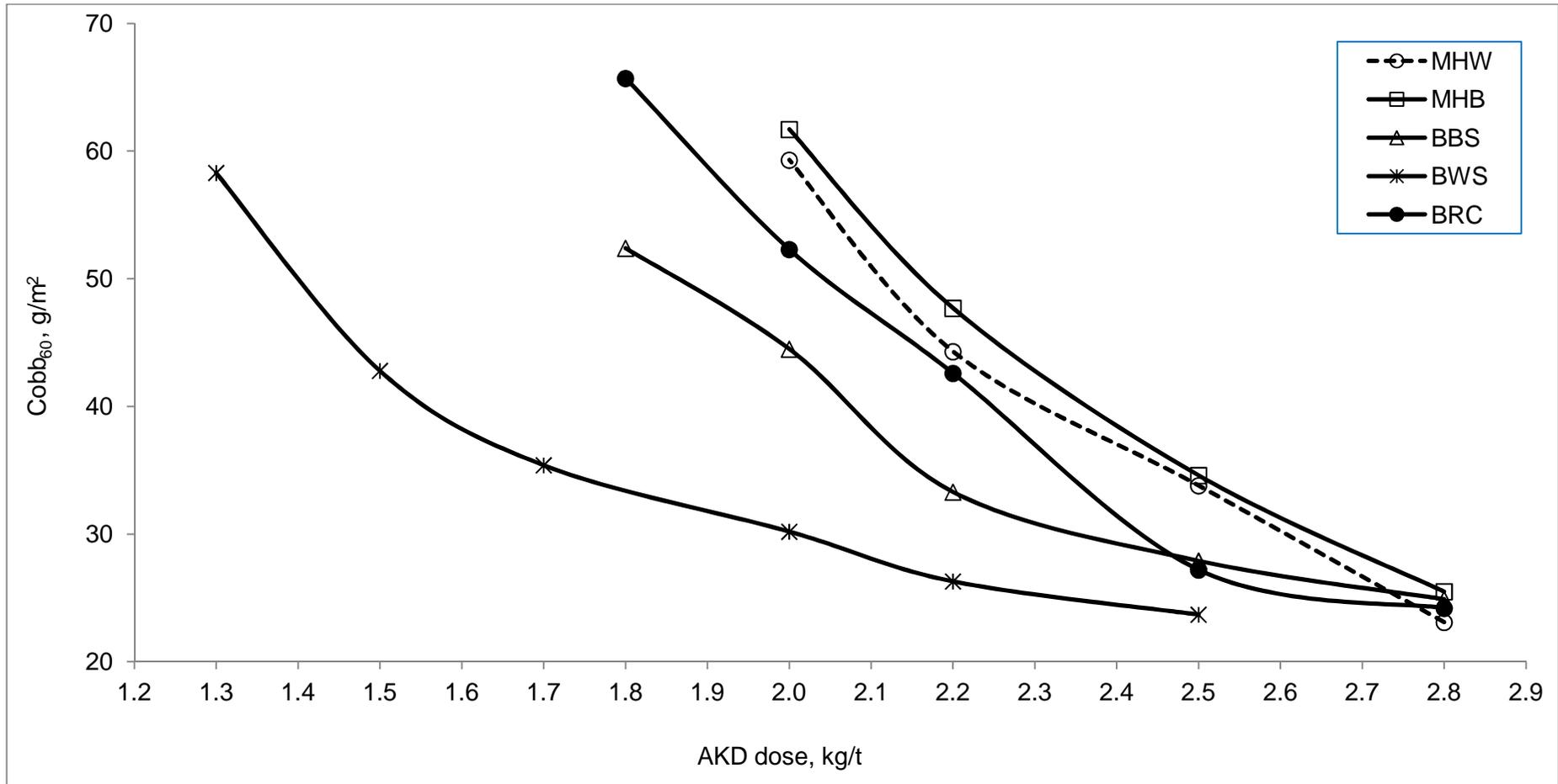
Figure 23: Comparison of Cobb<sub>60</sub> value of different pulp furnishes in AKD sizing with PCC filler
