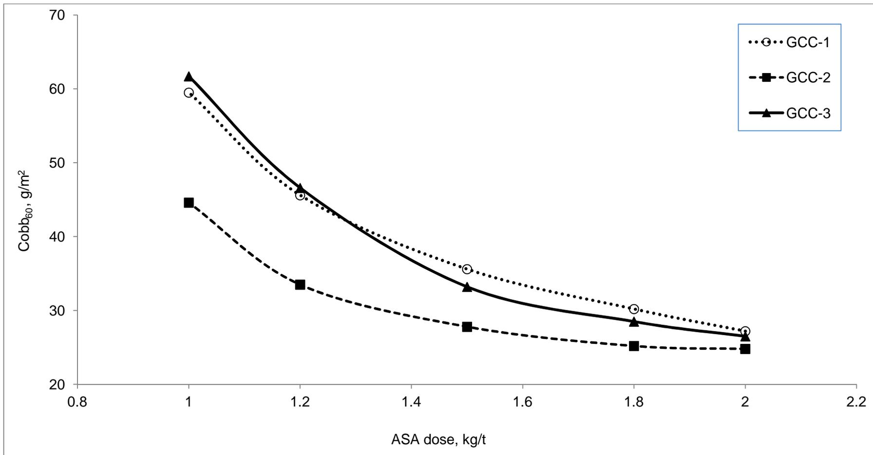
Figure 32: Sizing performance of different GCC fillers with MHB pulp in ASA sizing
