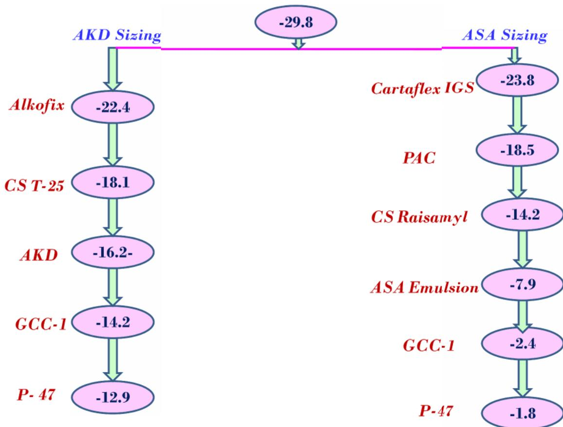
Fig:1 Study on charge demand of pulp stock at various stages during its preparation using different sizing agents
