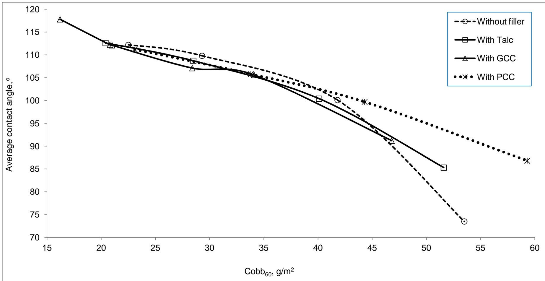
Figure 7: Cobb<sub>60</sub> vs. contact angle relationship for MHW pulp in AKD sizing
