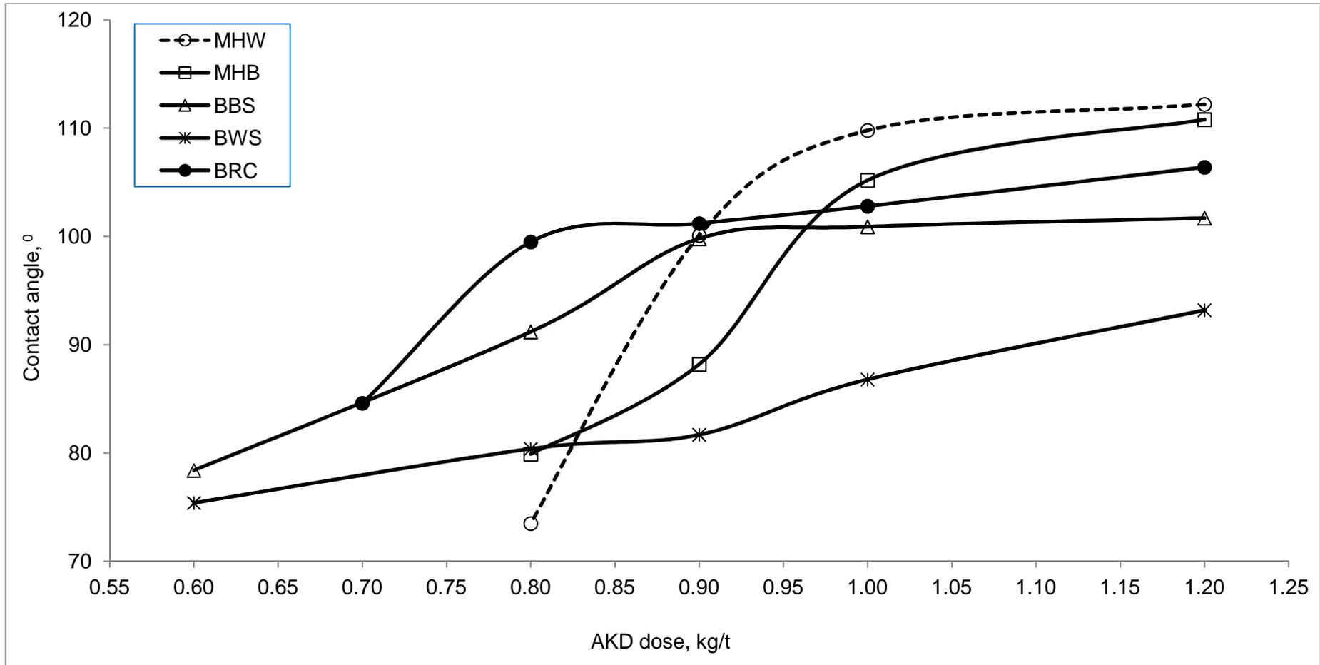
Figure 24: Comparison of contact angle of different pulp furnishes in AKD sizing (without filler)
