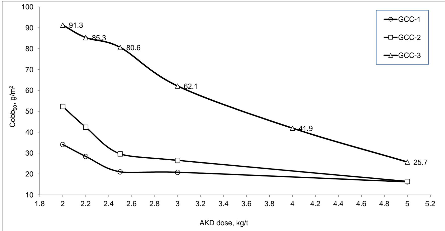
Figure 3: Effect of GCC filler on Cobb<sub>60</sub> value of paper made with MHW pulp in AKD sizing
