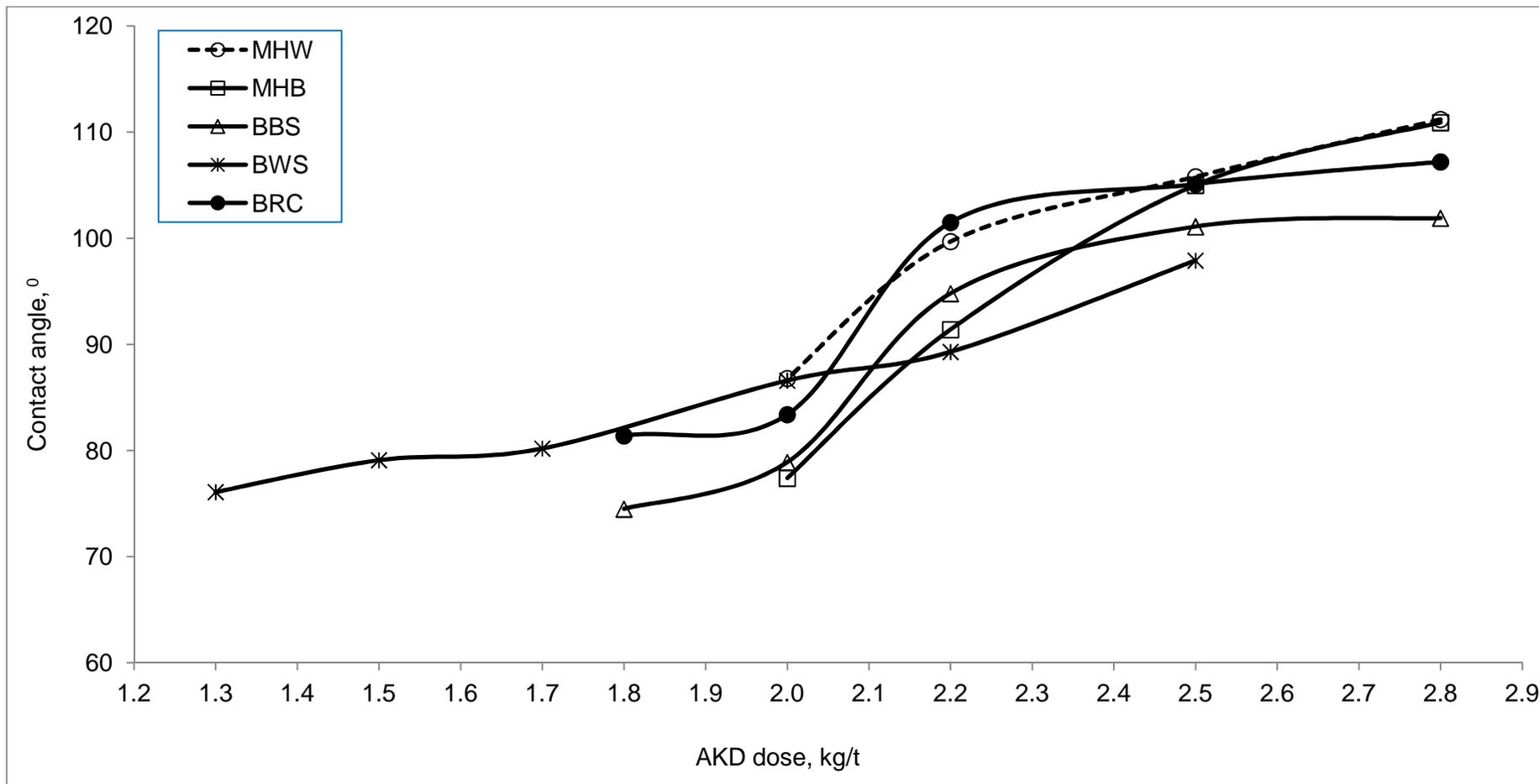
Figure 27: Comparison of contact angle of different pulp furnishes in AKD sizing with PCC filler
