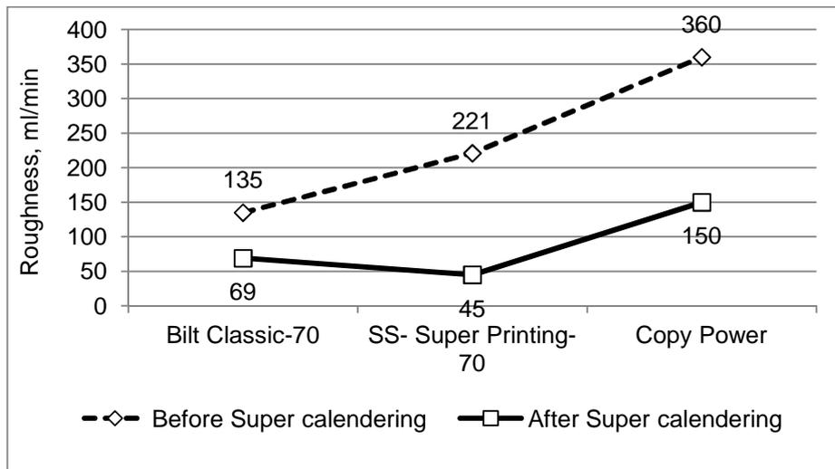
Figure 4. Effect of super calendering on felt side of paper
