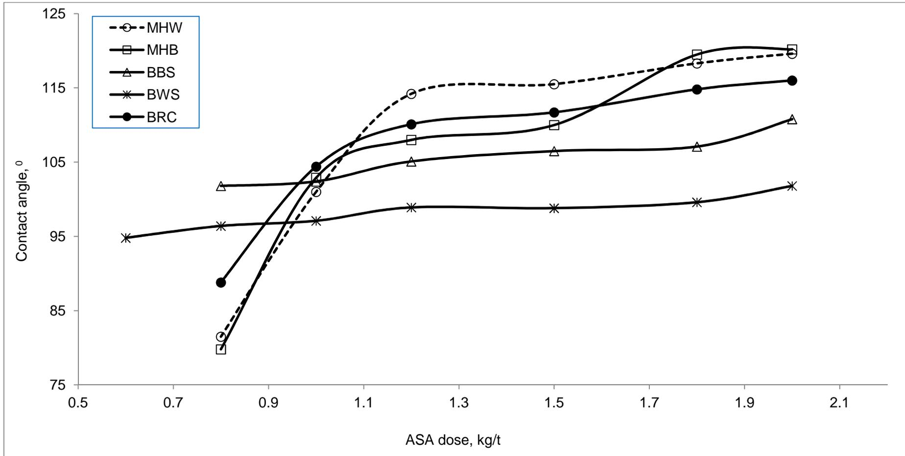
Figure 54: Comparison of contact angle of different pulp furnishes in ASA sizing with talc filler
