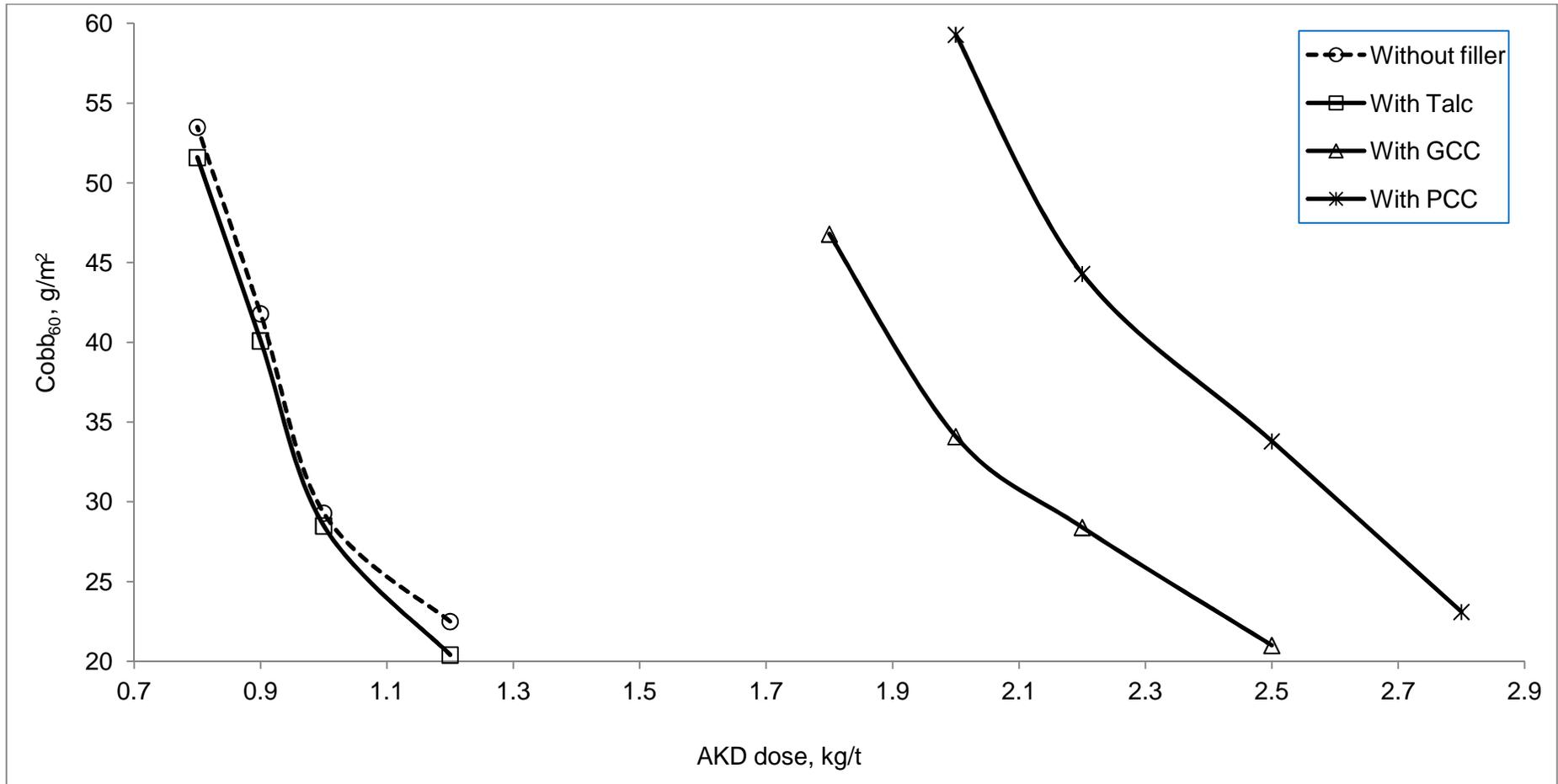
Figure 5: Effect of filler on Cobb<sub>60</sub> value with MHW pulp in AKD sizing
