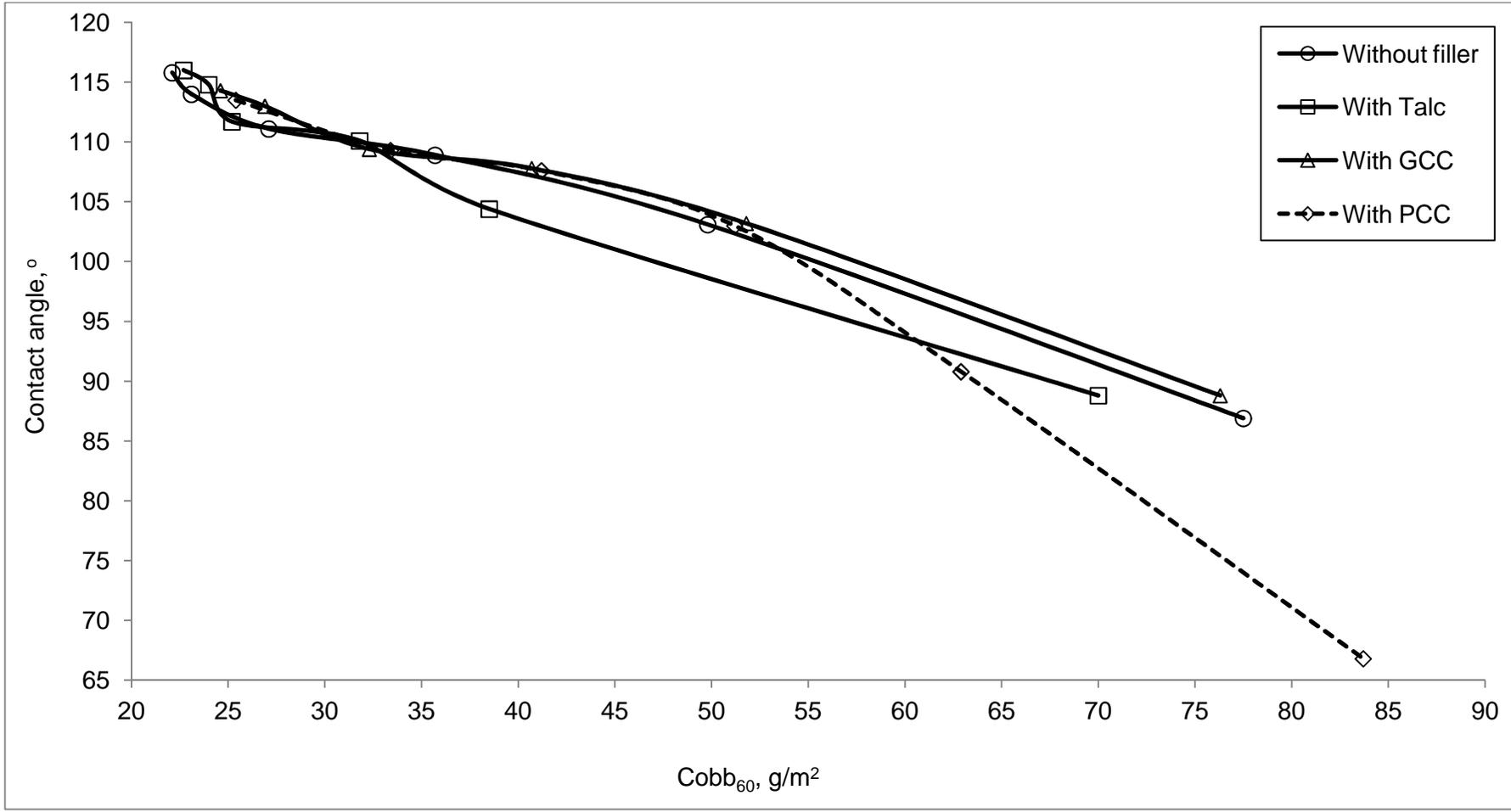
Table 48: Cobb<sub>60</sub> vs. contact angle relationship of BRC pulp in ASA sizing with different fillers
