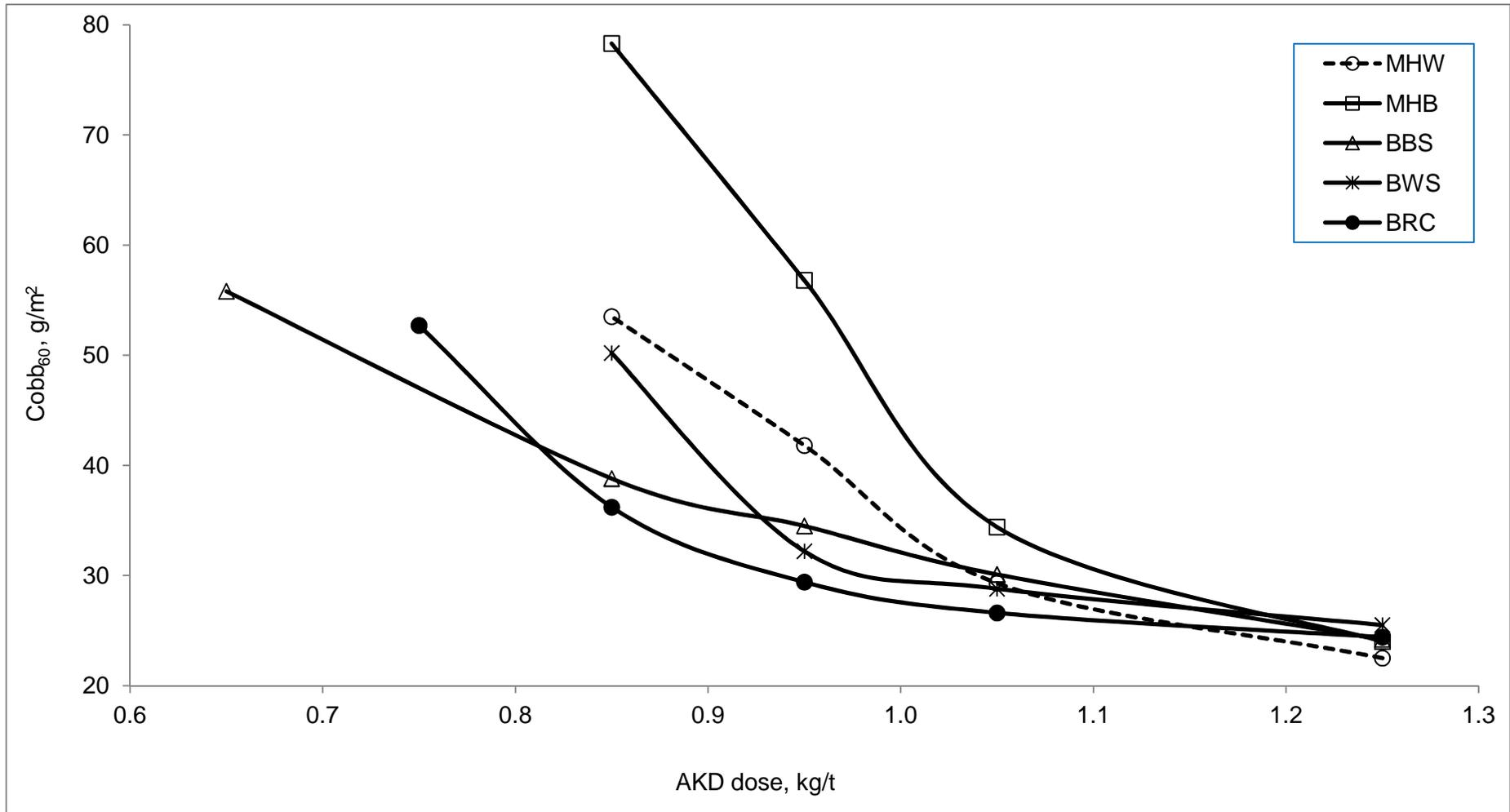
Figure 20: Comparison of Cobb<sub>60</sub> value of different pulp furnishes in AKD sizing (without filler)
