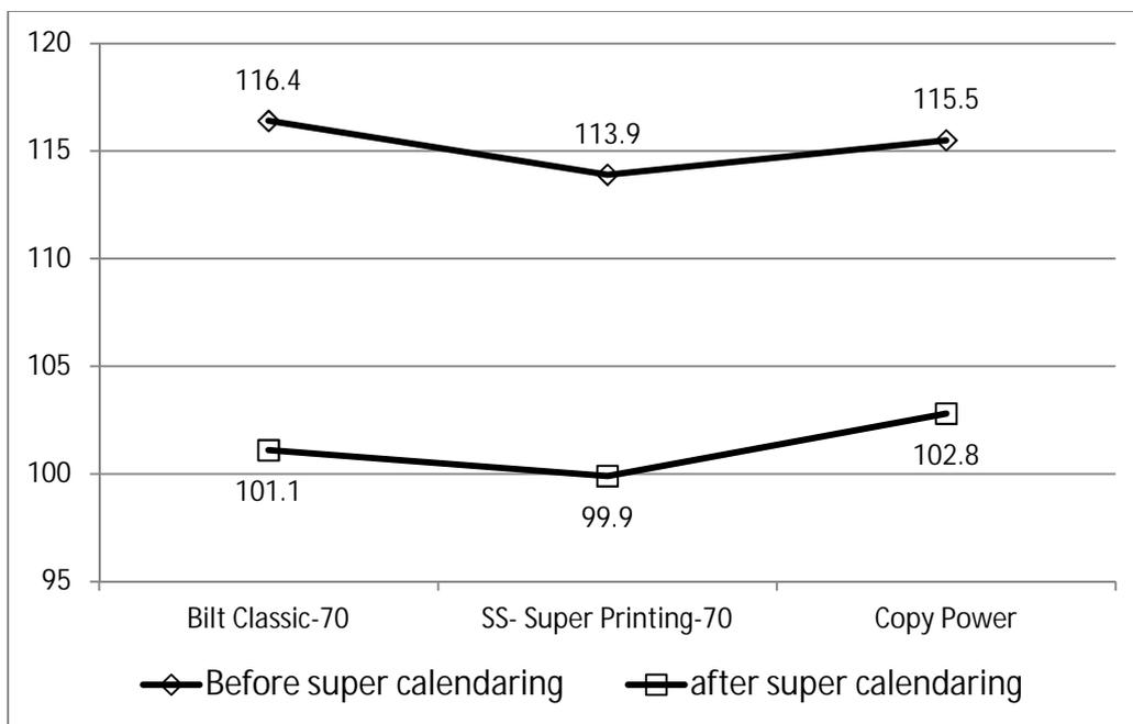
Figure 6. Effect of super calendering on contact angle of felt side of paper
