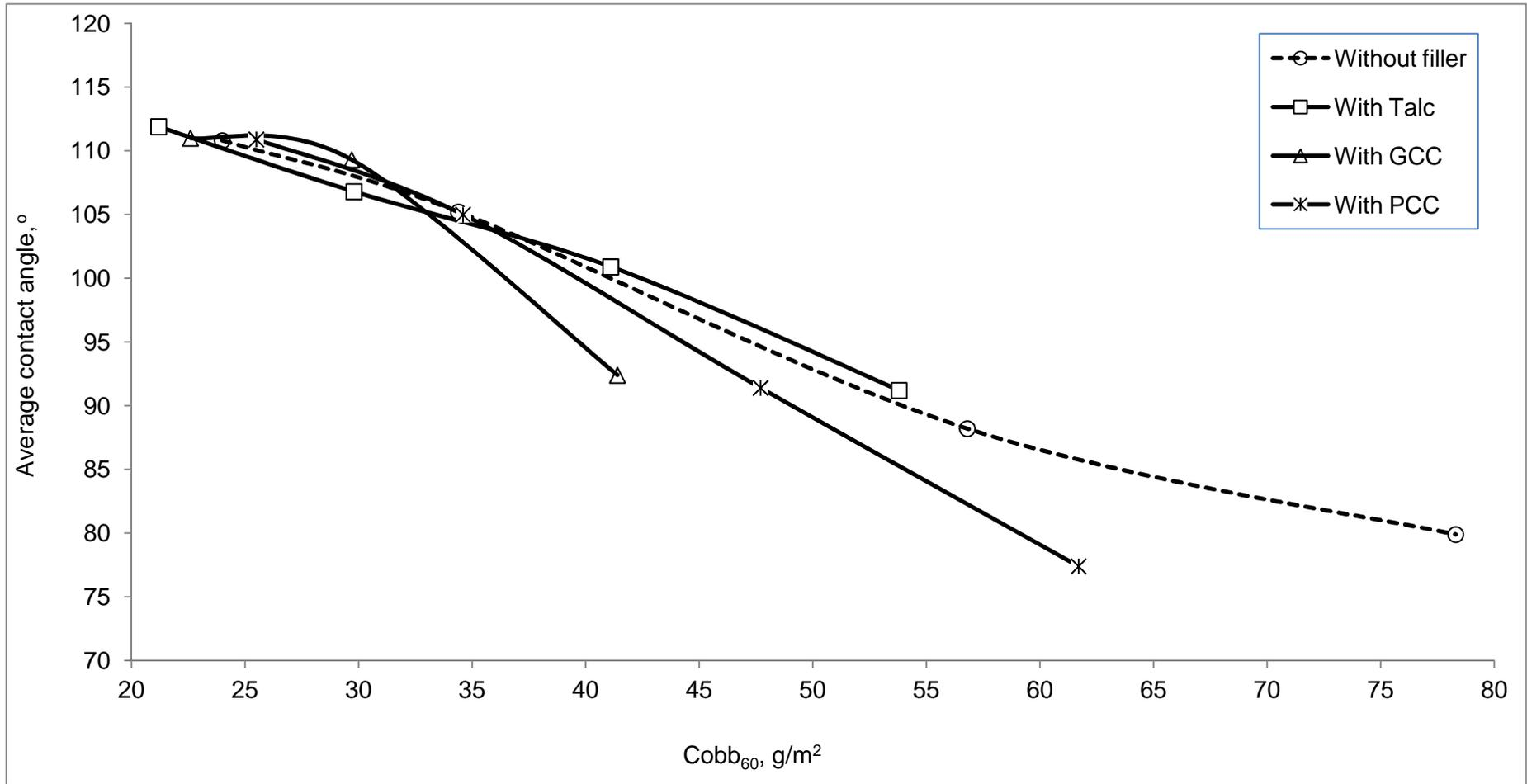
Figure 10: Cobb<sub>60</sub> vs. contact angle relationship for MHB pulp in AKD sizing
