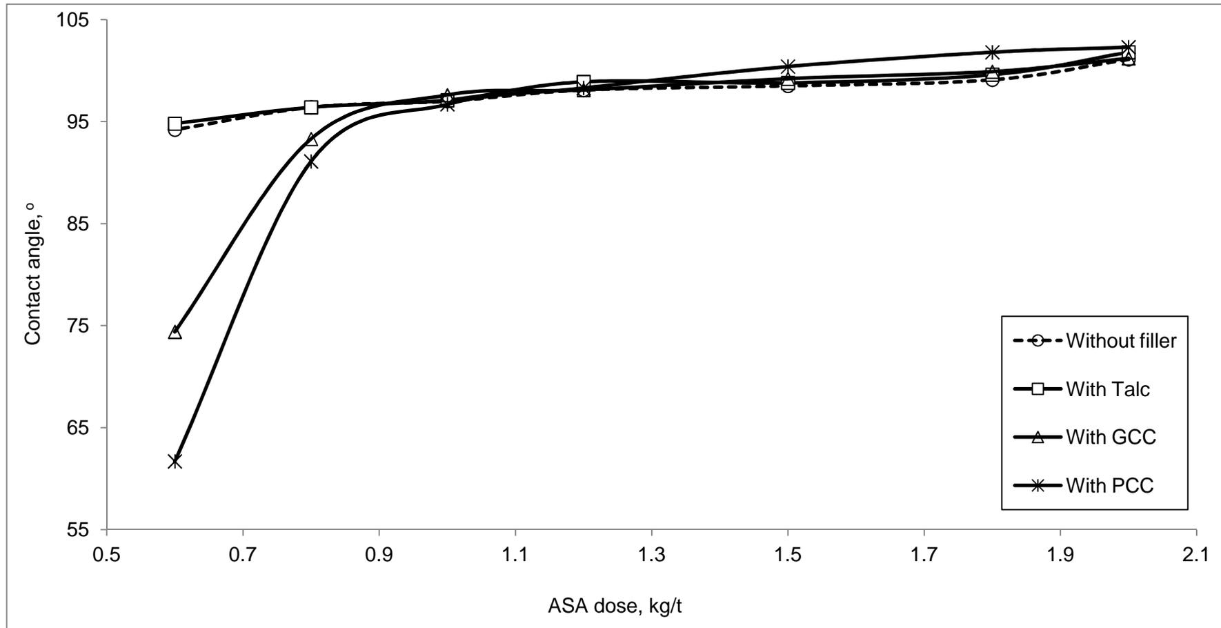
Figure 44: Effect of filler on contact angle with BWS pulp in ASA sizing
