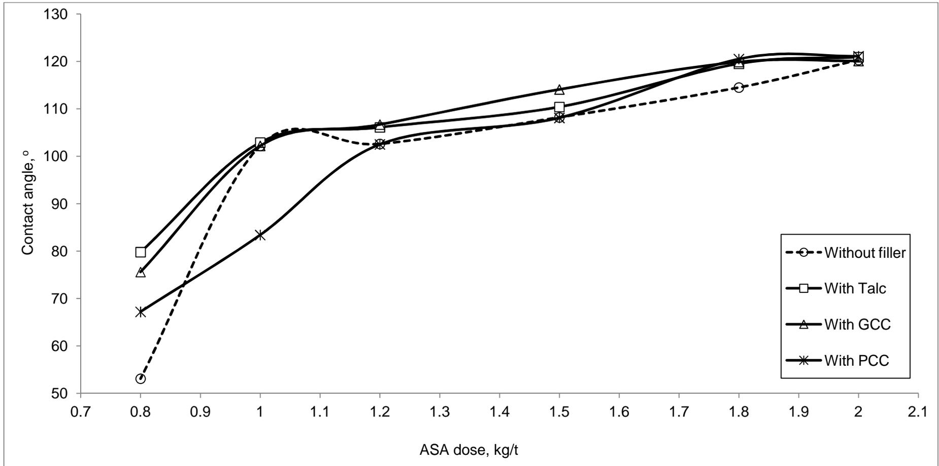
Figure 35: Effect of filler on contact angle with MHB pulp in ASA sizing
