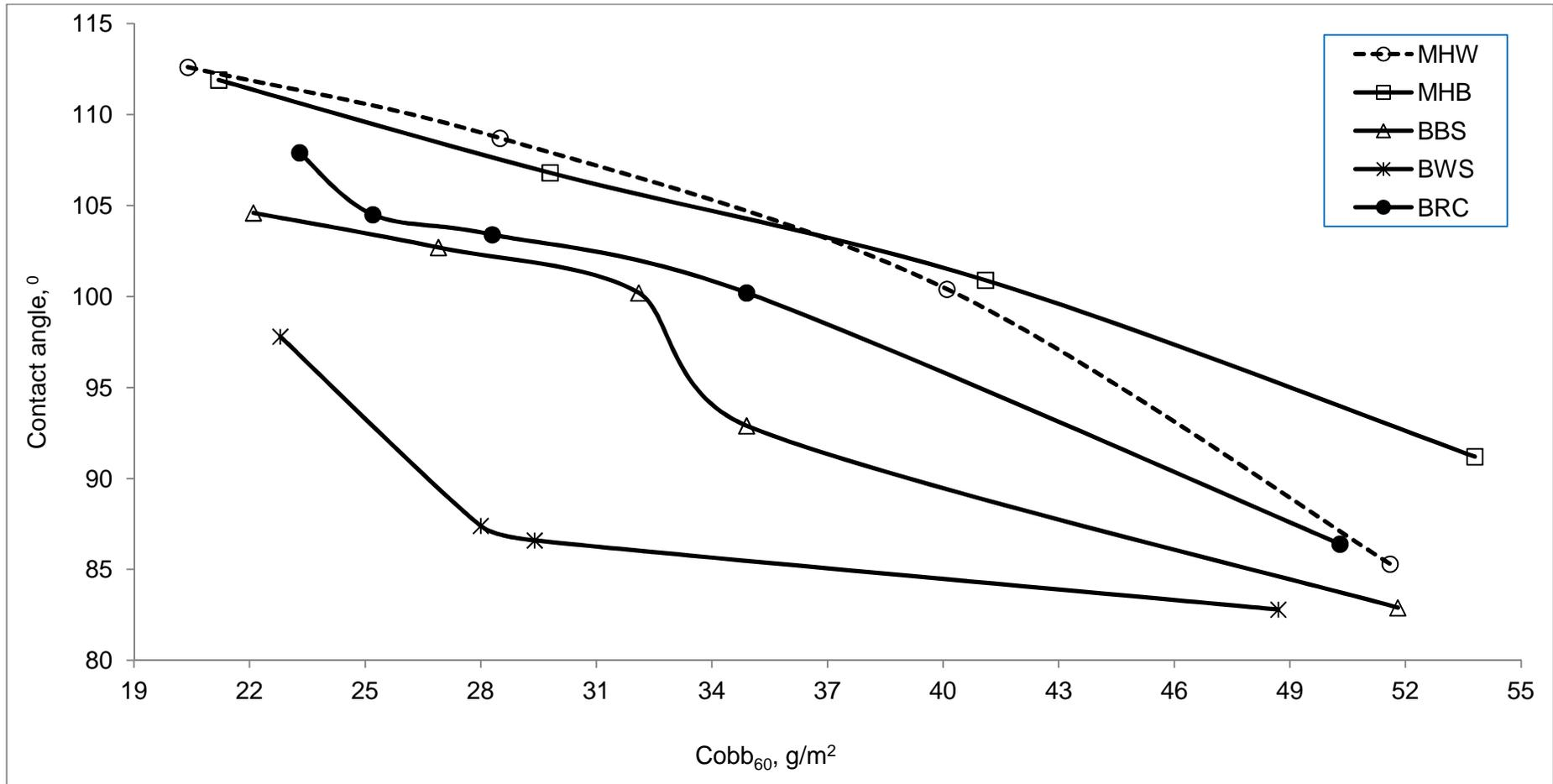
Figure 29: Cobb vs. contact angle relationship for different pulp furnishes in AKD sizing with talc filler
