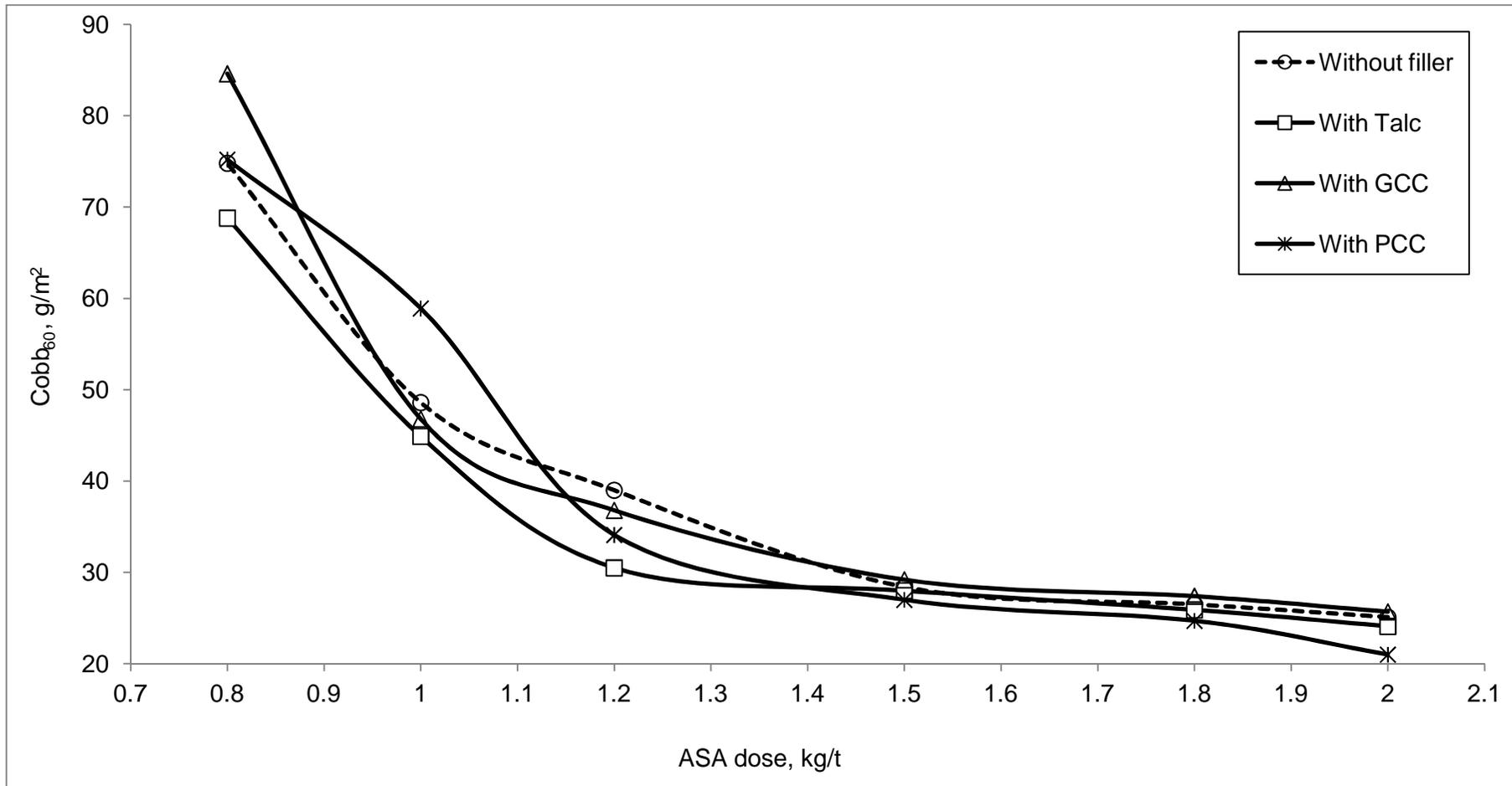
Figure 37: Effect of filler on Cobb<sub>60</sub> value with MHW pulp in ASA sizing
