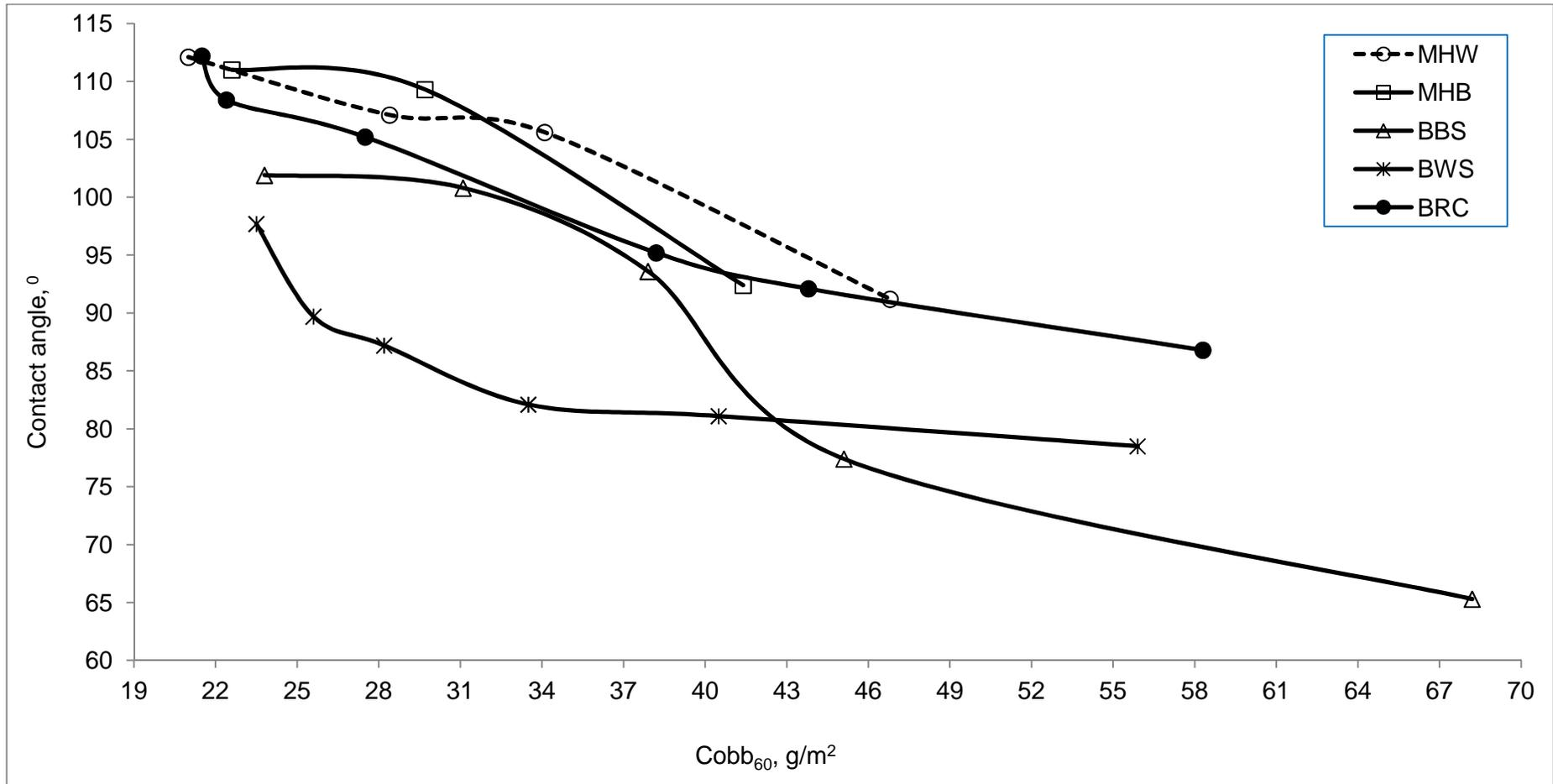
Figure 30: Cobb vs. contact angle relationship for different pulp furnishes in AKD sizing with GCC filler
