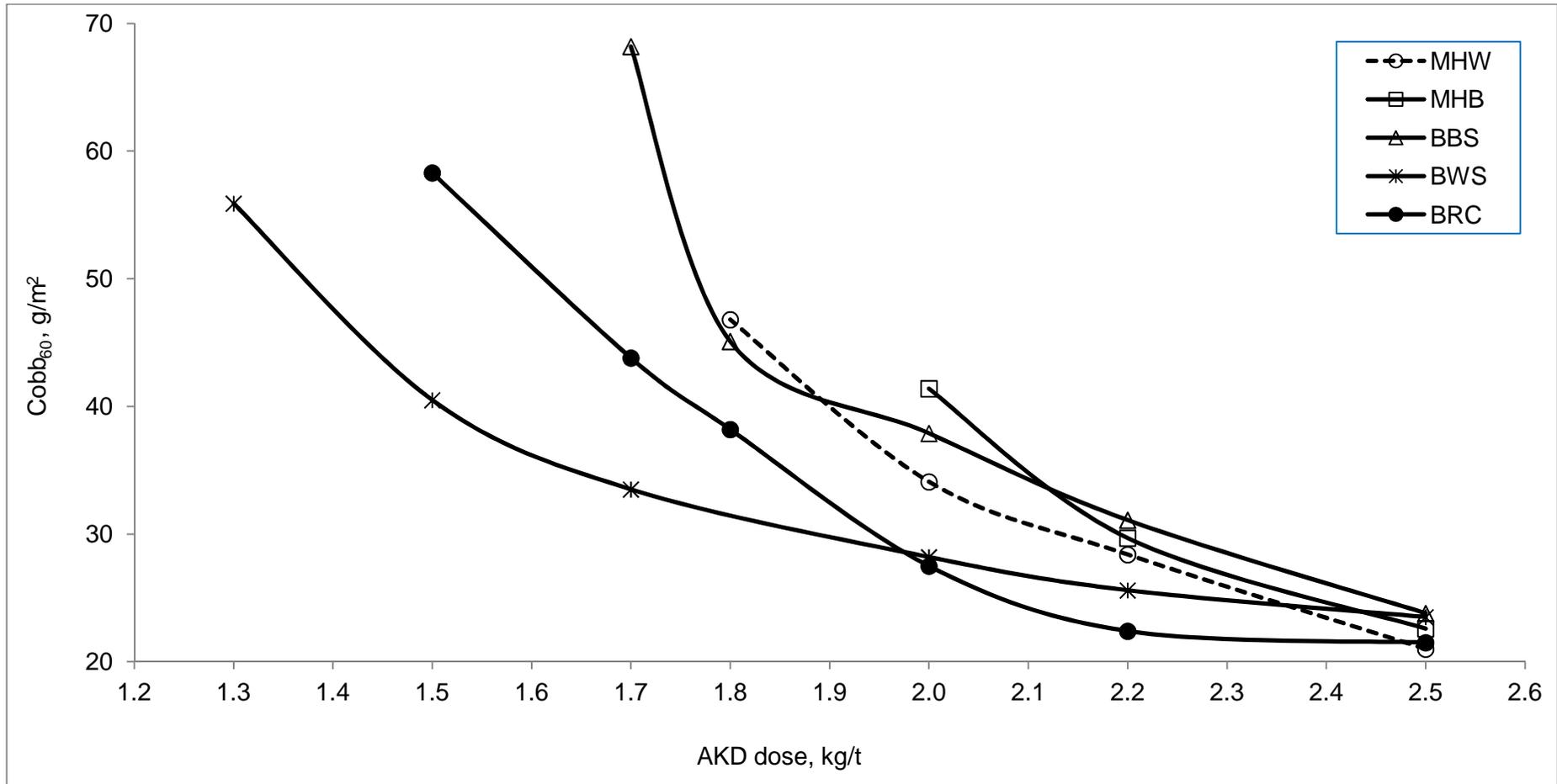
Figure 22: Comparison of Cobb<sub>60</sub> value of different pulp furnishes in AKD sizing with GCC filler
