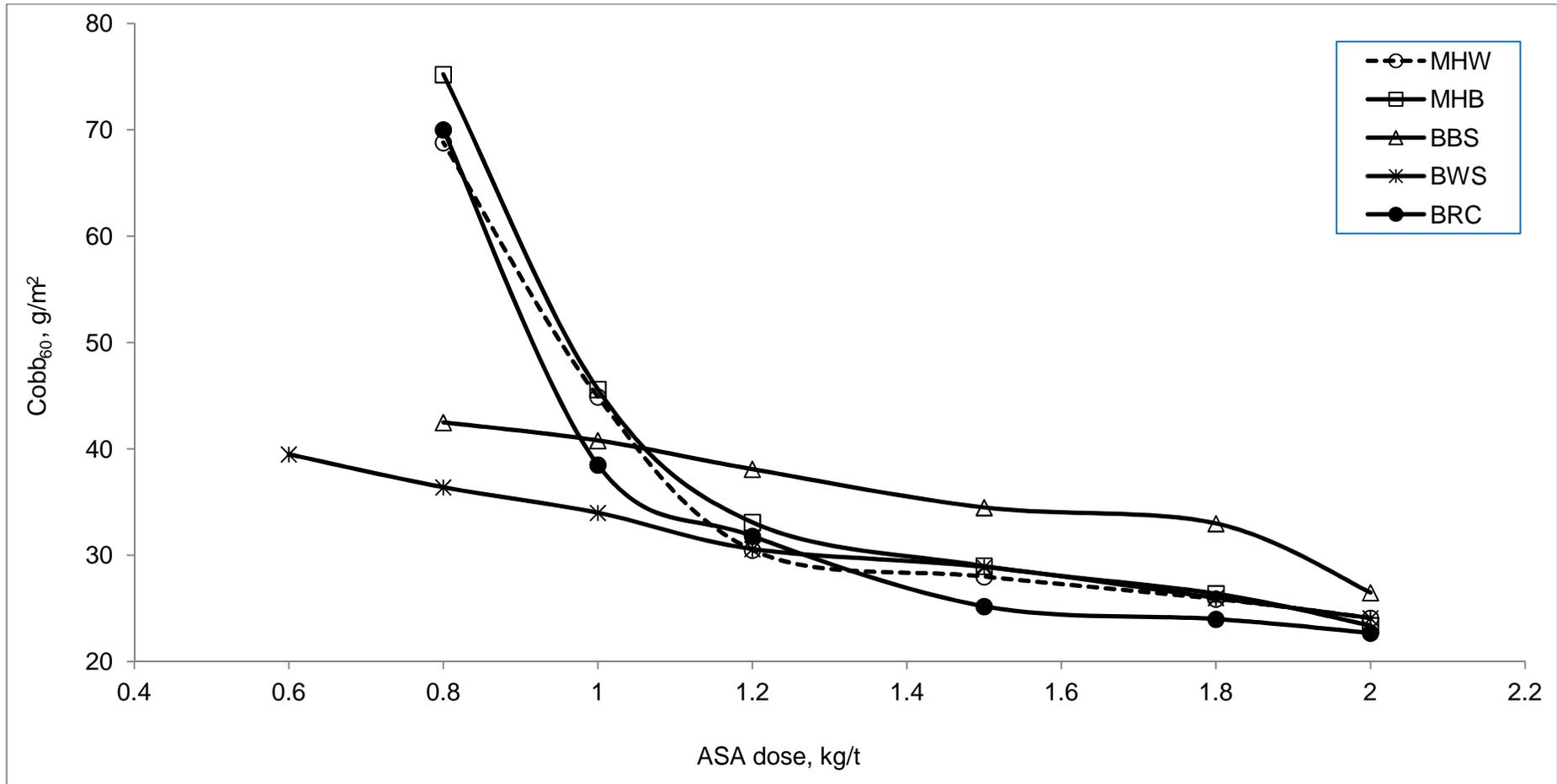
Figure 50: Comparison of Cobb<sub>60</sub> value of different pulp furnishes in ASA sizing with talc filler
