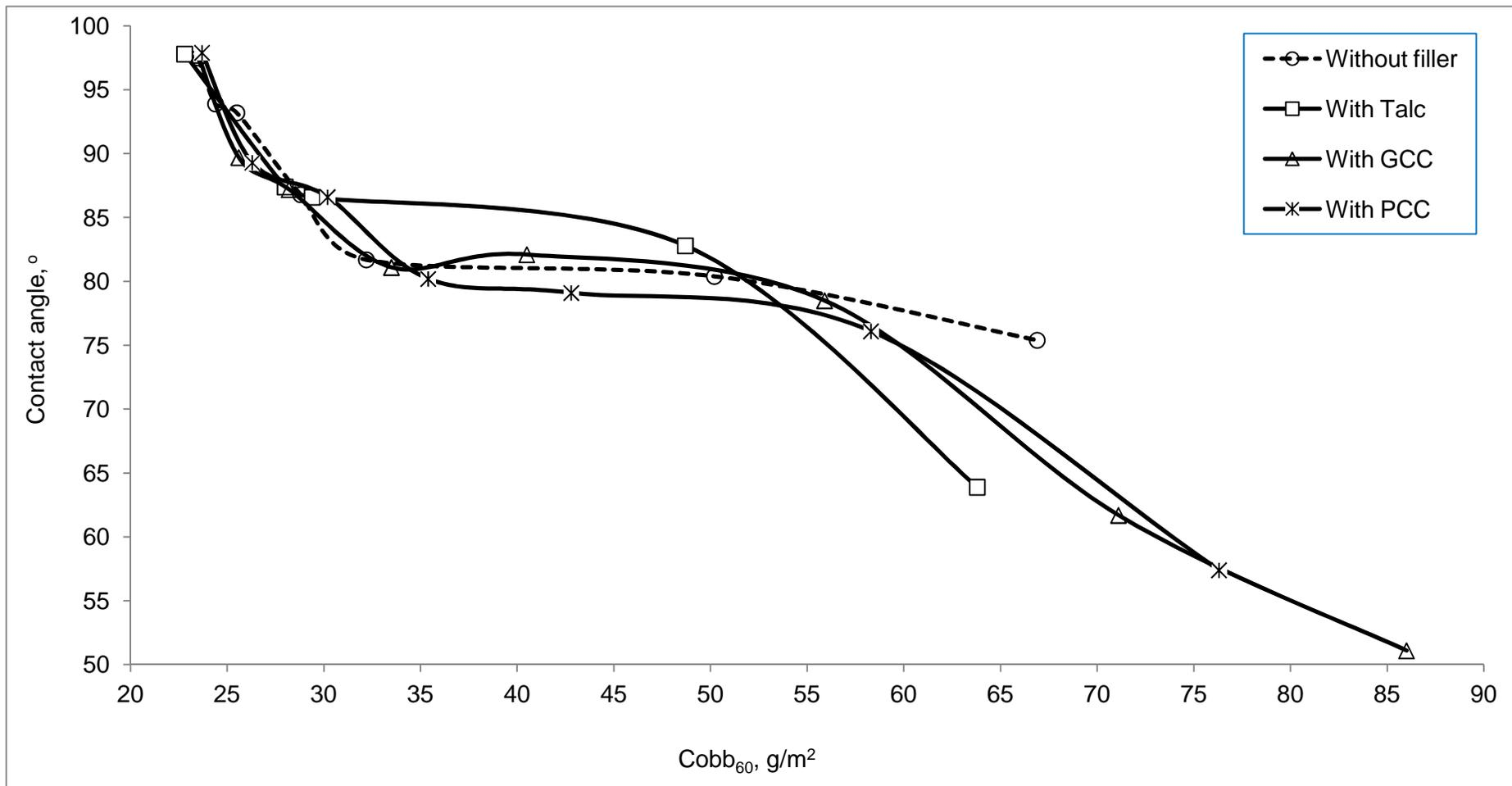
Figure 16: Cobb<sub>60</sub> vs. contact angle relationship for BWS pulp in AKD sizing
