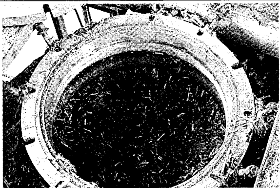
Fig 10. Pulping Digester filled with jute chips
