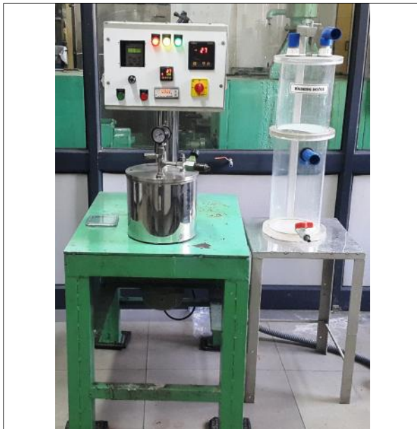
Oxygen bleaching reactor
