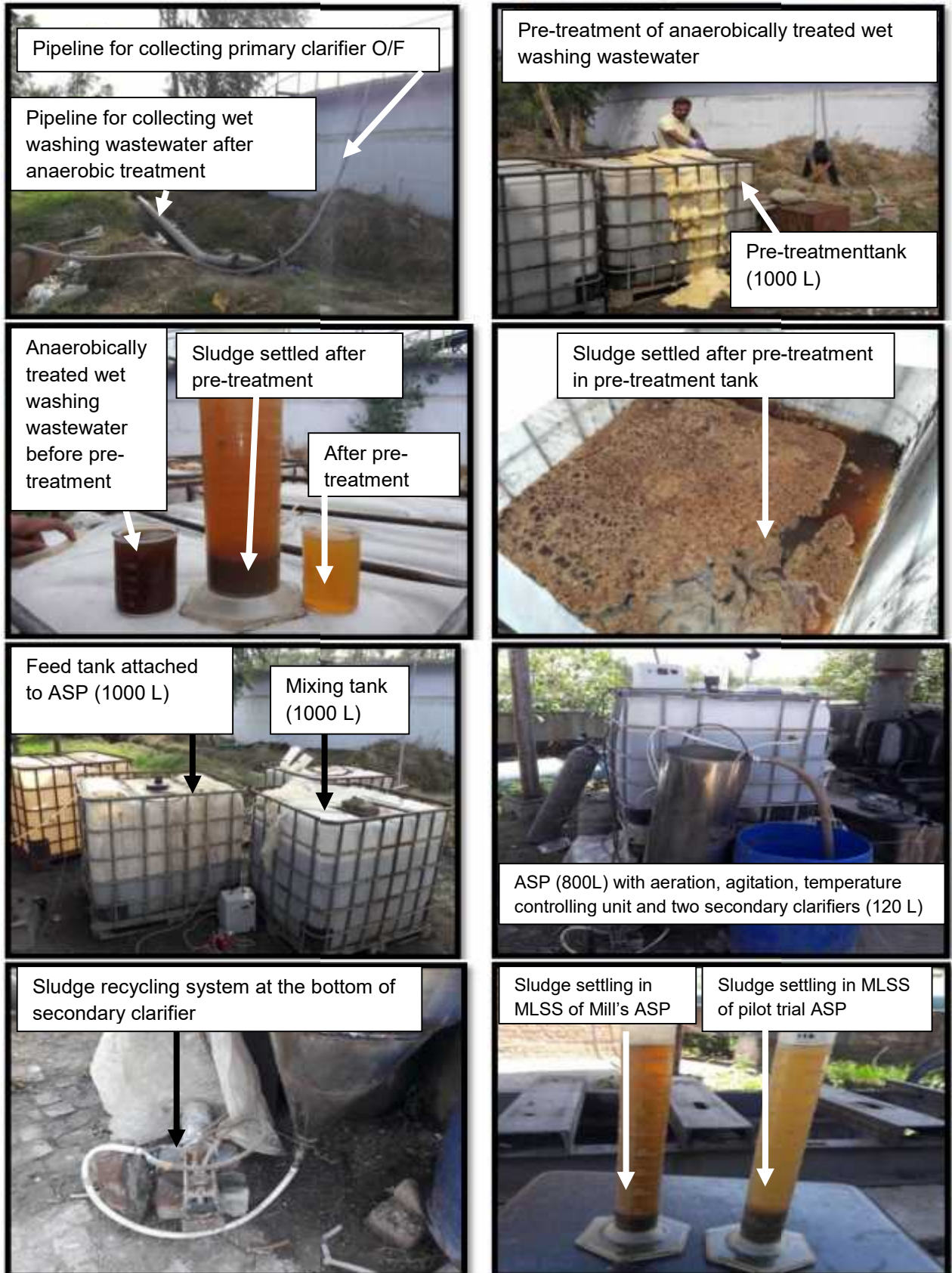
Figure 16: Pilot scale ( 1.15 \text{ m}^3/\text{day} ) set up for wastewater treatment at mill site
